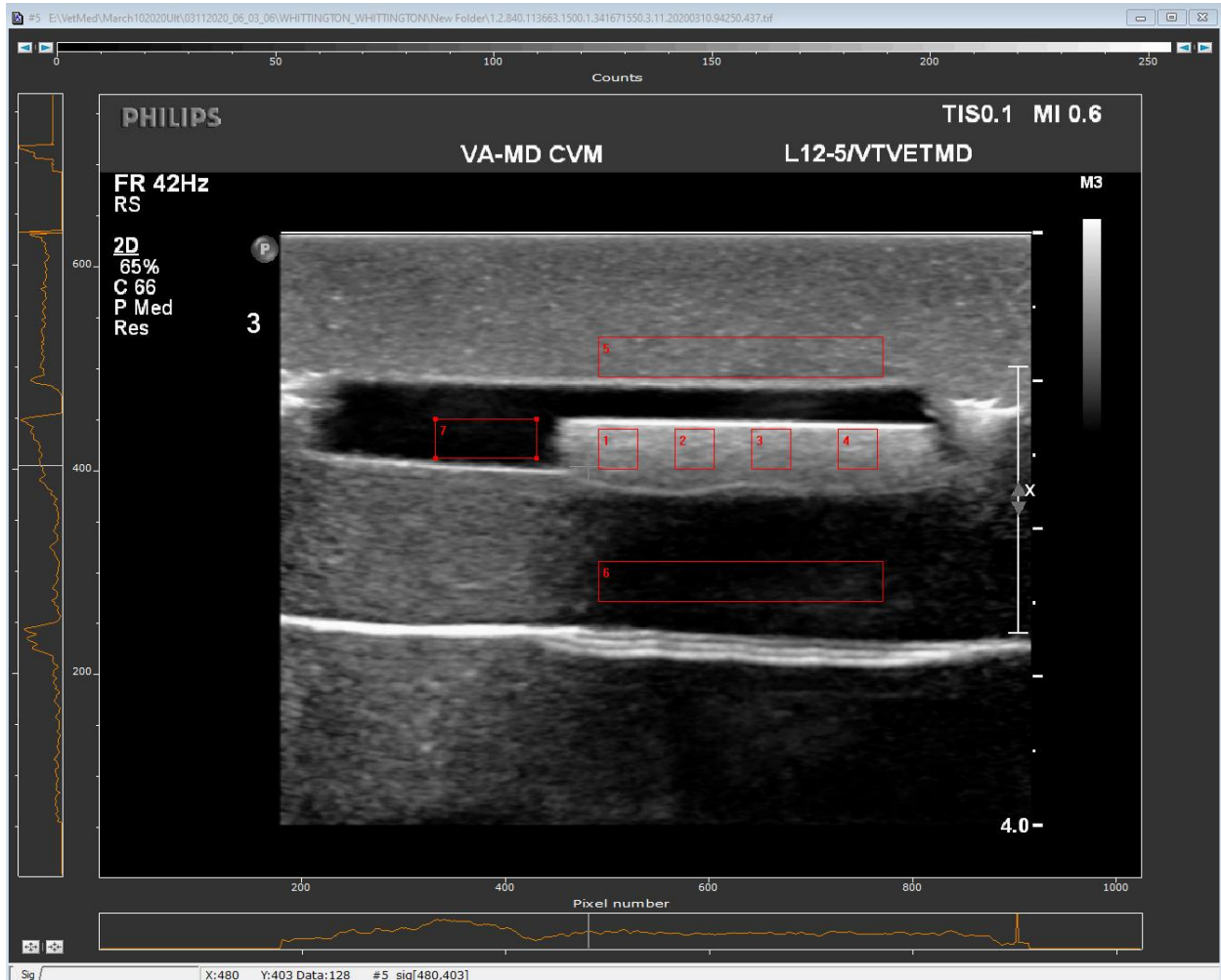
Figure S1: B-Mode images of a 3 wt%P40 Sample under 12MHz ultrasound imaging, analyzed for Signal-to-Noise ratio, using Andor Solis software, and containing four areas of interest defined throughout the sample (1-4). Box 5 & 6 were used to compare Signal-to-noise of the gelatin mimic, while box 7 compared dI water SNR (Data not shown).
