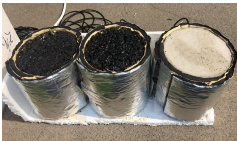
Figure 2. Wrapped specimens with side and bottom thermal insulated (left: dense asphalt concrete or AC13; middle: porous asphalt concrete or PAC13; right: cement concrete or C25).
