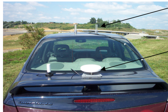
Figure 14: DGPS and DSRC Antennas
