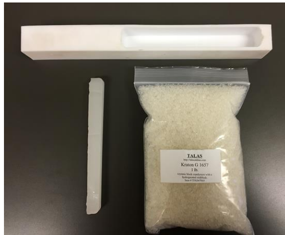
Figure 4-19 Mold for TPE pellets (top), molded TPE (left) and TPE pellets (right)
