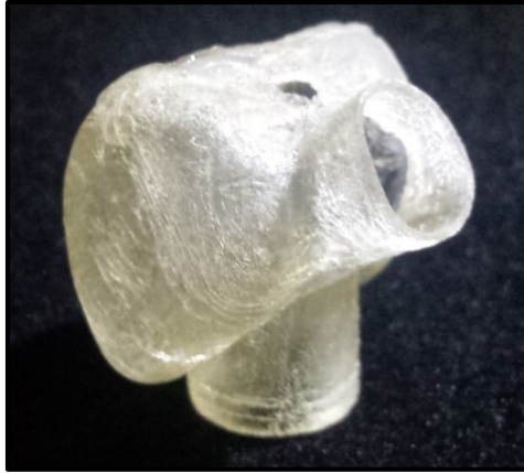
Figure 87 - 3D printed nectophore, showing thin wall structure and stress fractures along the shell periphery.
