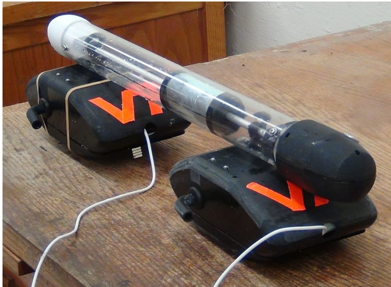
Figure 135 – Example of a multi-jet colonial robot with deployable units, constructed by a senior design class team in conjunction with the siphonophore robot project. Lower power pumps forced water through frontal scoops to jet out of nozzles that could be vectored for 3D motion. The units were designed to reduce drag, stabilize roll, and attach and reattach with a central stem.
