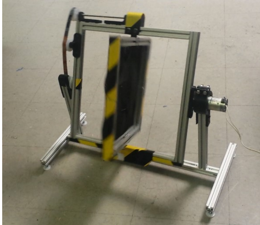
Figure 88 - Custom built rotocasting frame with two degree of freedom motion
