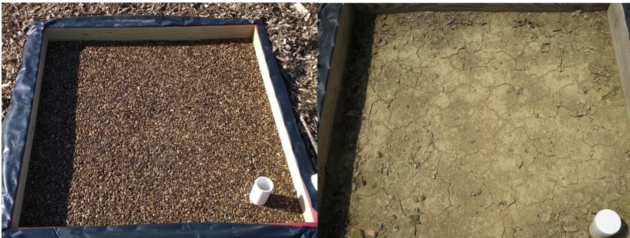
Fig. S5. Photographs of finished surface for PP (left) and UP tree pits showing albedo contrast between treatments at the Mountain site.
