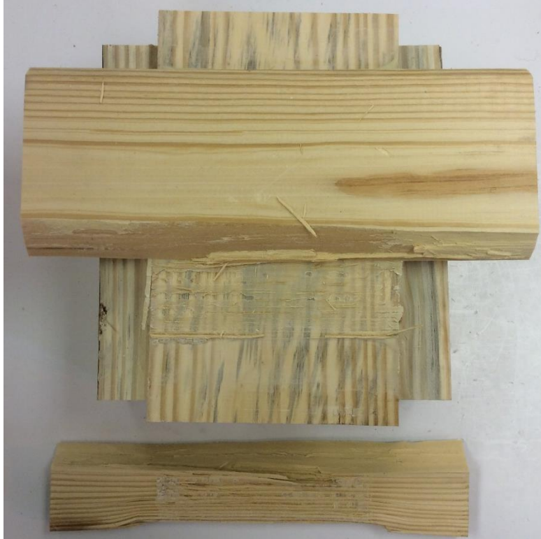
Lower amount of wood failure for samples made with the solvent based construction adhesive (SBCA) and tested in shear with compression failure
