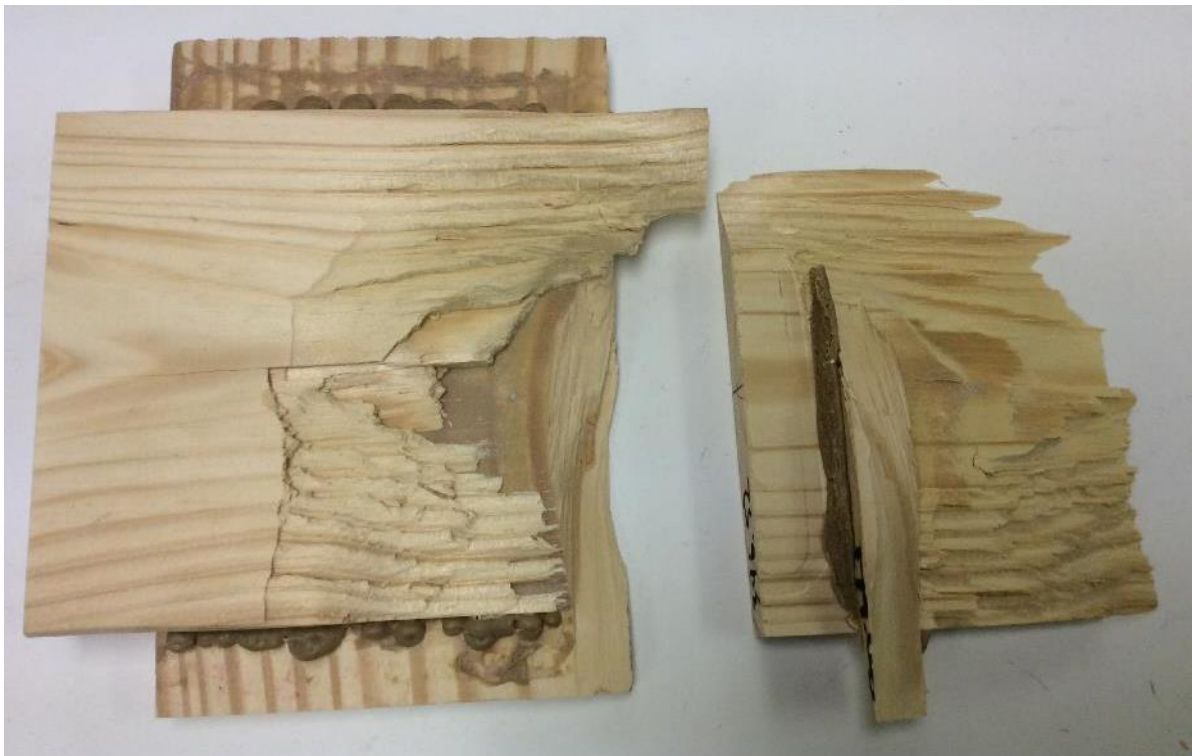
High amounts of wood failure for samples made with the solvent based construction adhesive (SBCA) and tested in tension perpendicular to the grain
