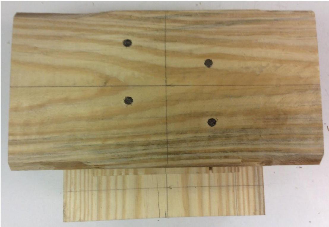
Top view of failure of nailed samples tested in shear
