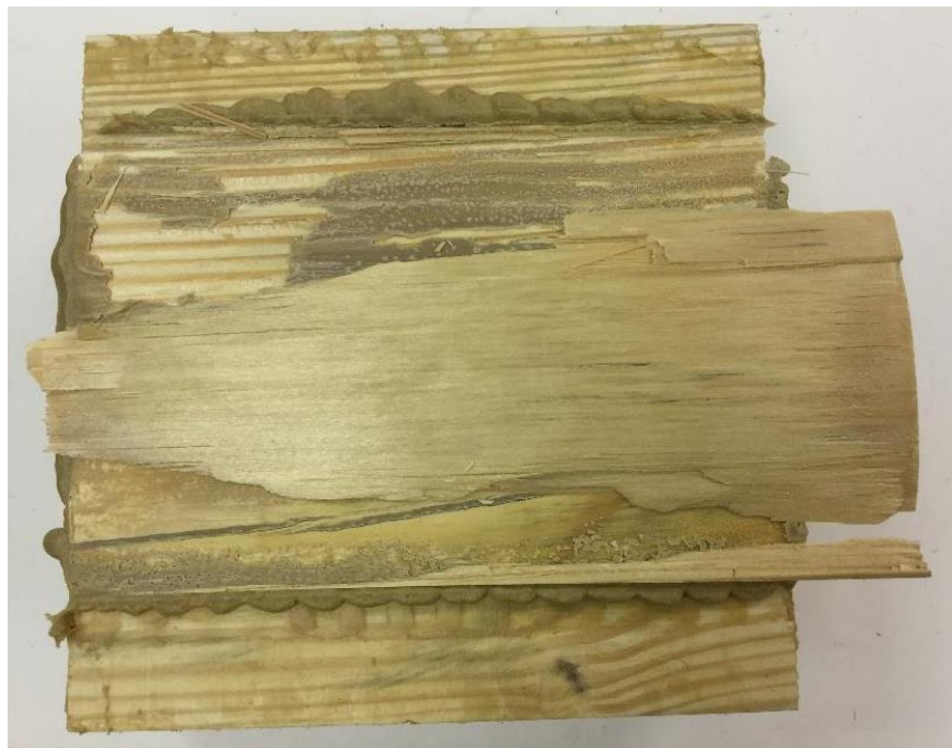
High amounts of wood failure for samples made with the solvent based construction adhesive (SBCA) and tested in tension parallel to the grain
