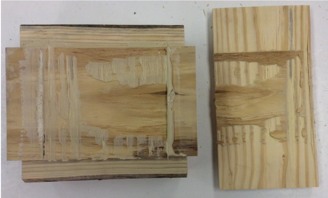
Low amount of wood failure for samples made with the emulsion polymer isocyanate (EPI) and tested in shear with shear failure
