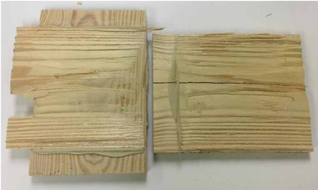
High amounts of wood failure made with the emulsion polymer isocyanate (EPI) and tested in tension perpendicular to the grain
