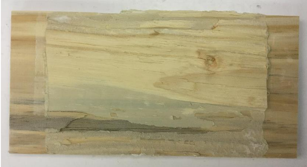
Low amounts of wood failure made with the emulsion polymer isocyanate (EPI) and tested in tension parallel to the grain
