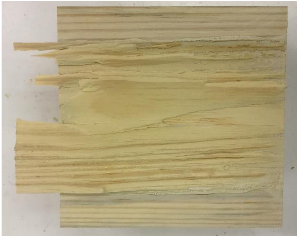
High amounts of wood failure made with the emulsion polymer isocyanate (EPI) and tested in tension parallel to the grain
