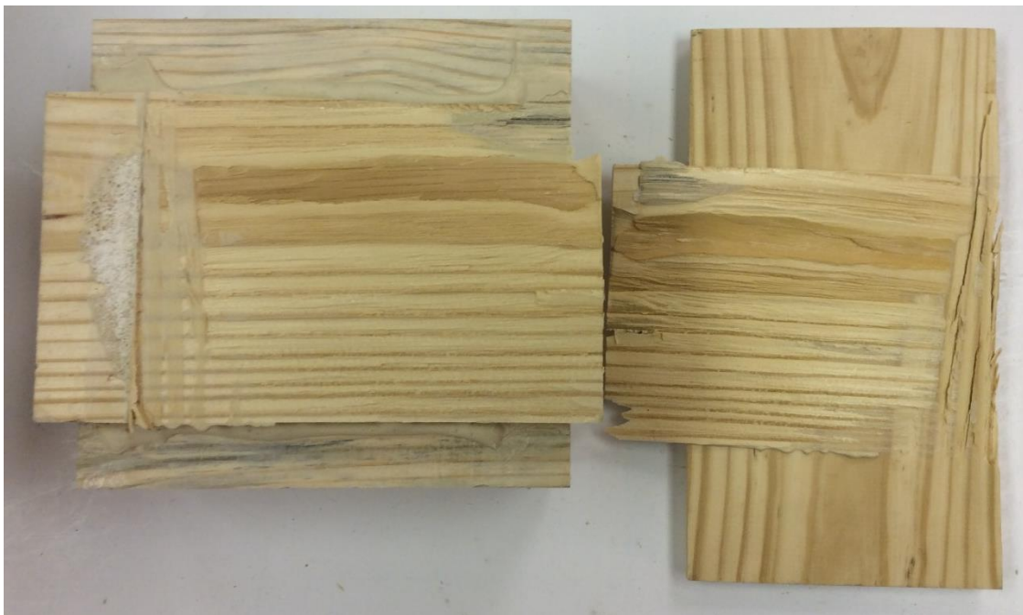
High amount of wood failure for samples made with the emulsion polymer isocyanate (EPI) and tested in shear with shear failure
