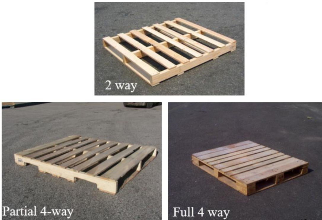
Figure 4. Photographs of two-way entry stringer pallet (top), partial four-way entry stringer pallet (bottom left), and four-way entry block pallet (bottom right)
