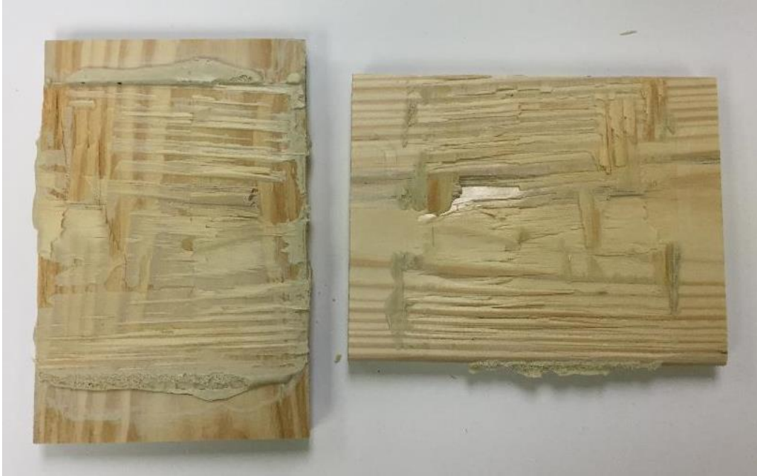
Low amounts of wood failure for samples made with the emulsion polymer isocyanate (EPI) and tested in tension perpendicular to the grain
