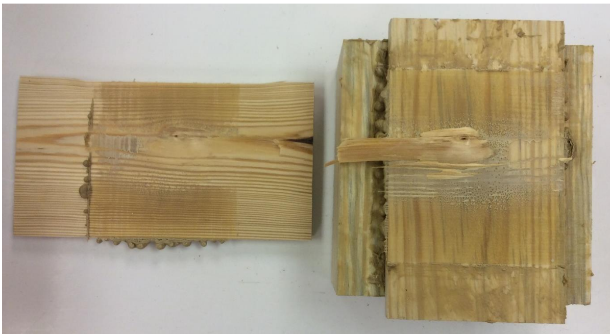
Higher amount of wood failure for samples made with the solvent based construction adhesive (SBCA) and tested in shear with shear failure
