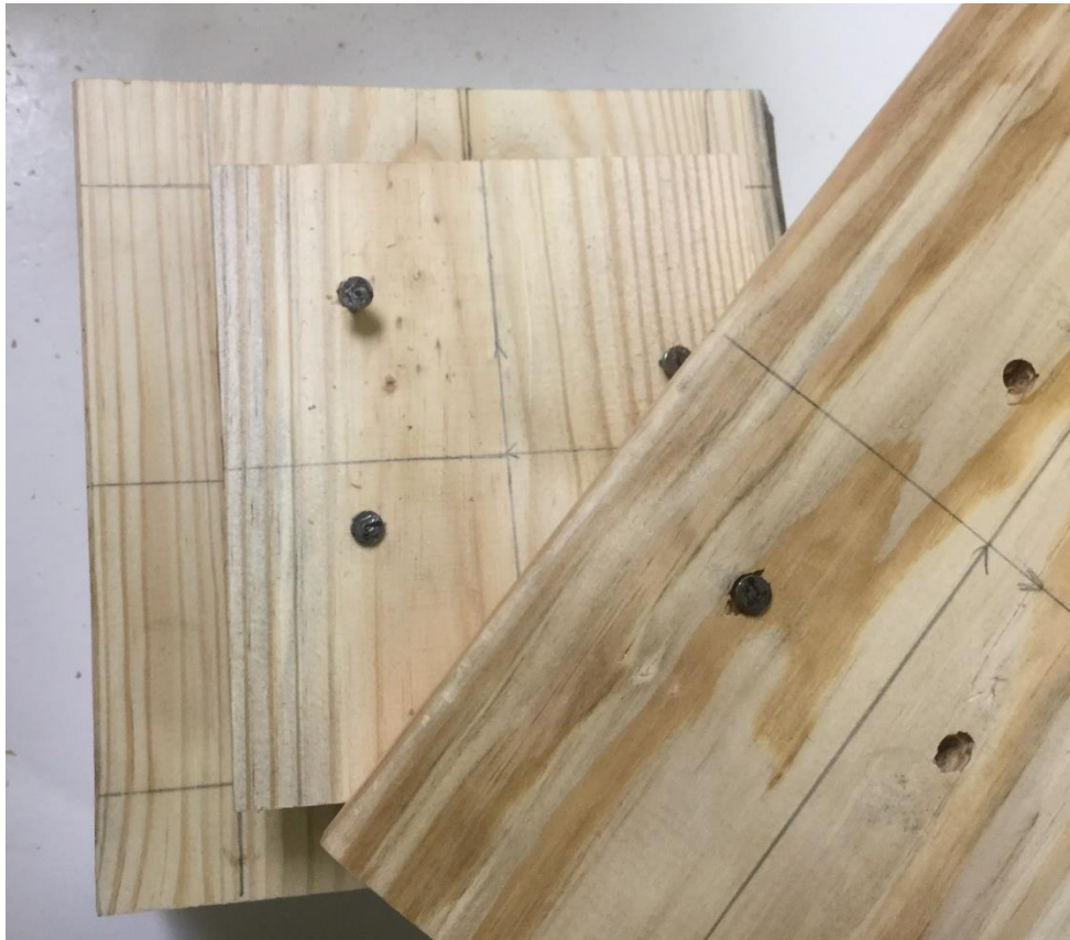
Top view of withdrawal failure of nailed samples tested in tension
