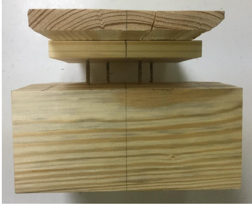
Side view of withdrawal failure of nailed samples tested in tension
