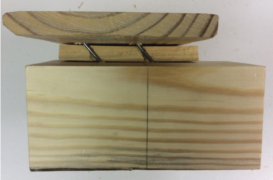
Side view of failure of nailed samples tested in shear
