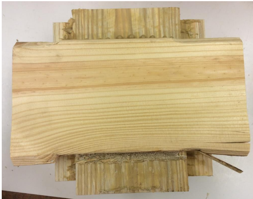
Higher amount of wood failure for samples made with the solvent based construction adhesive (SBCA) and tested in shear with compression failure
