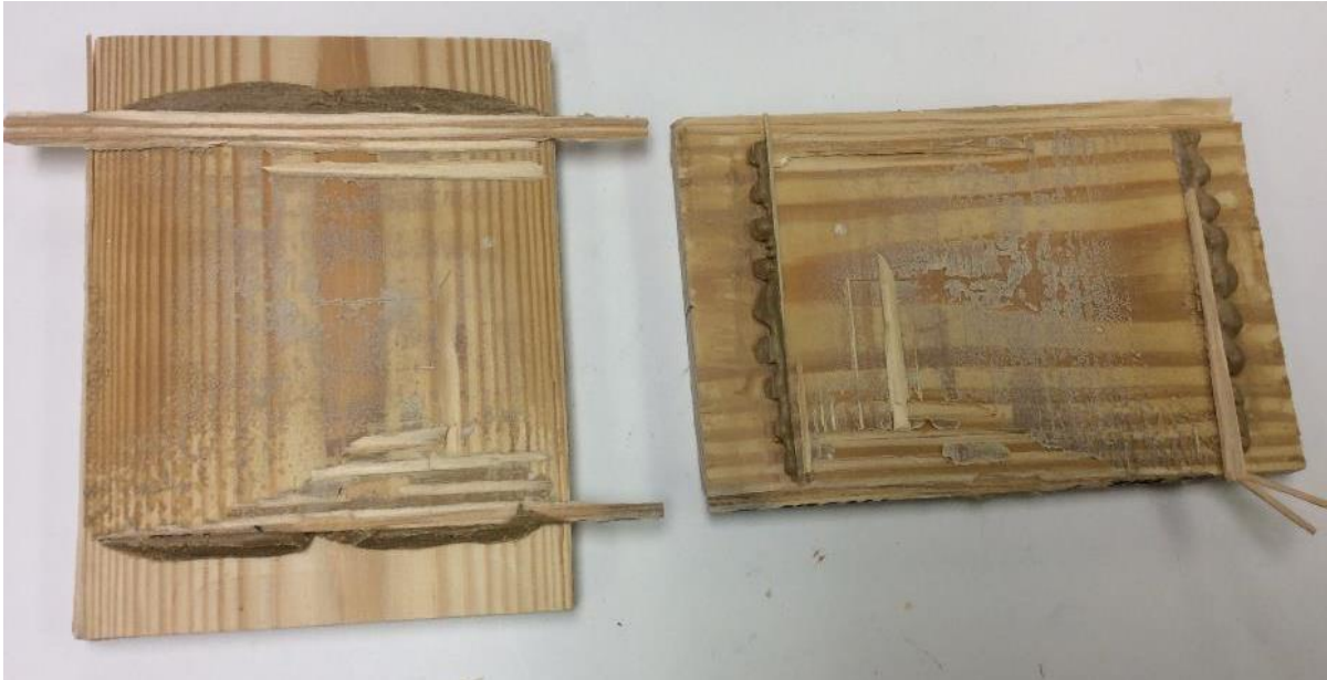
Low amounts of wood failure for samples made with the solvent based construction adhesive (SBCA) and tested in tension perpendicular to the grain
