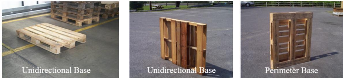
Figure 3. photographs of a unidirectional block pallet (left), unidirectional notched stringer pallet (middle), and perimeter block pallet (right)
