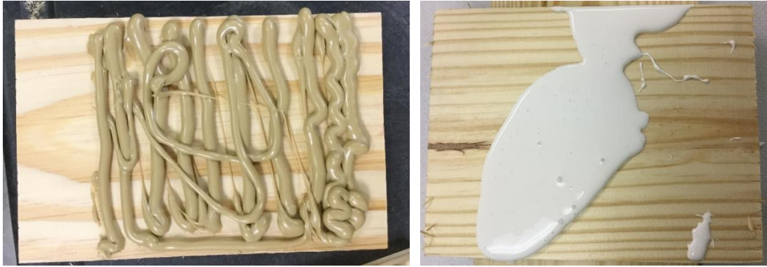
Figure 13. Example picture of the application of the two adhesives prior to spreading: (left) solvent based construction adhesive (SBCA), (right) emulsion polymer isocyanate (EPI).
