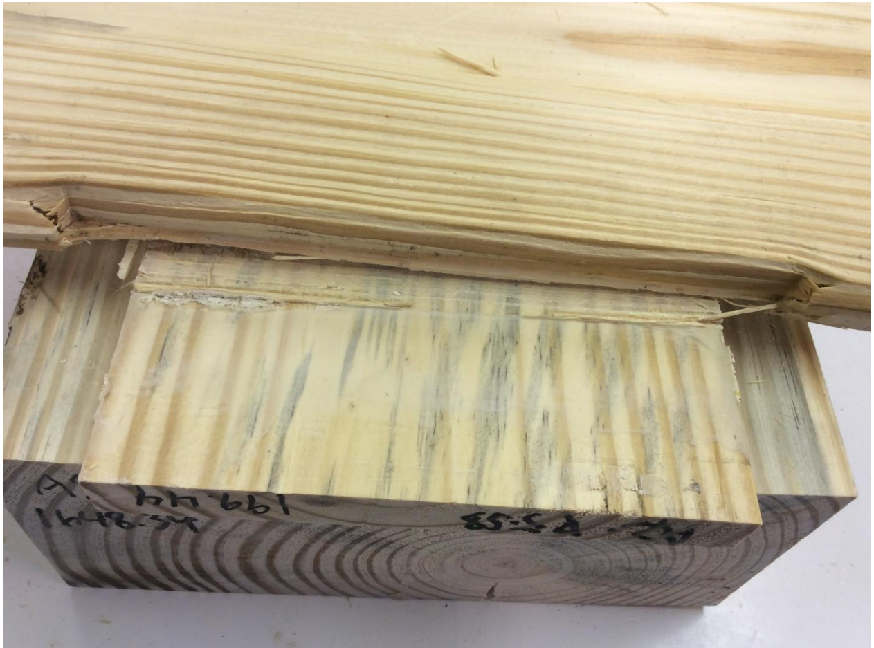
Wood failure for samples made with the emulsion polymer isocyanate (EPI) and tested in shear with compression failure
