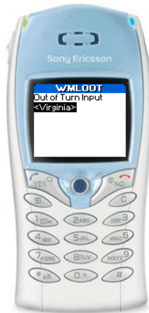
Figure 4.5: WMLOOT, an interaction interface for wireless devices within the WS://IM framework, as seen in a Sony Ericsson T68i.
