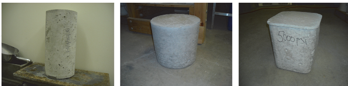
Figure 11. Types of concrete targets used for penetration testing.
