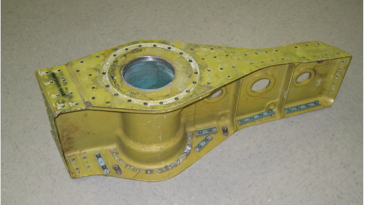
Figure 4.7. Aircraft rib supplied by United States Air Force
