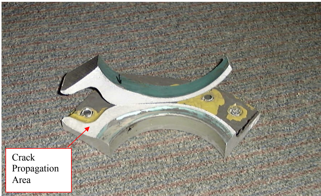
Figure 4.10. Section of aircraft rib that failed from fatigue
