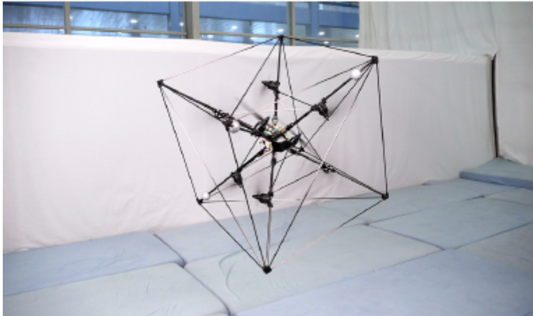
Figure 3.2: Omnicopter vehicle, designed by Brescianini and D'Andrea, fully assembled. Adapted from [2].
