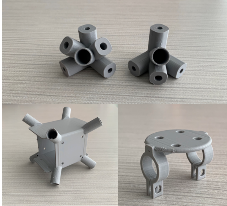
Figure 4.5: 3D printed Omnicopter parts. Top: The two variants of the corner bracket design. Left: The center housing design. Right: The motor clip design.
