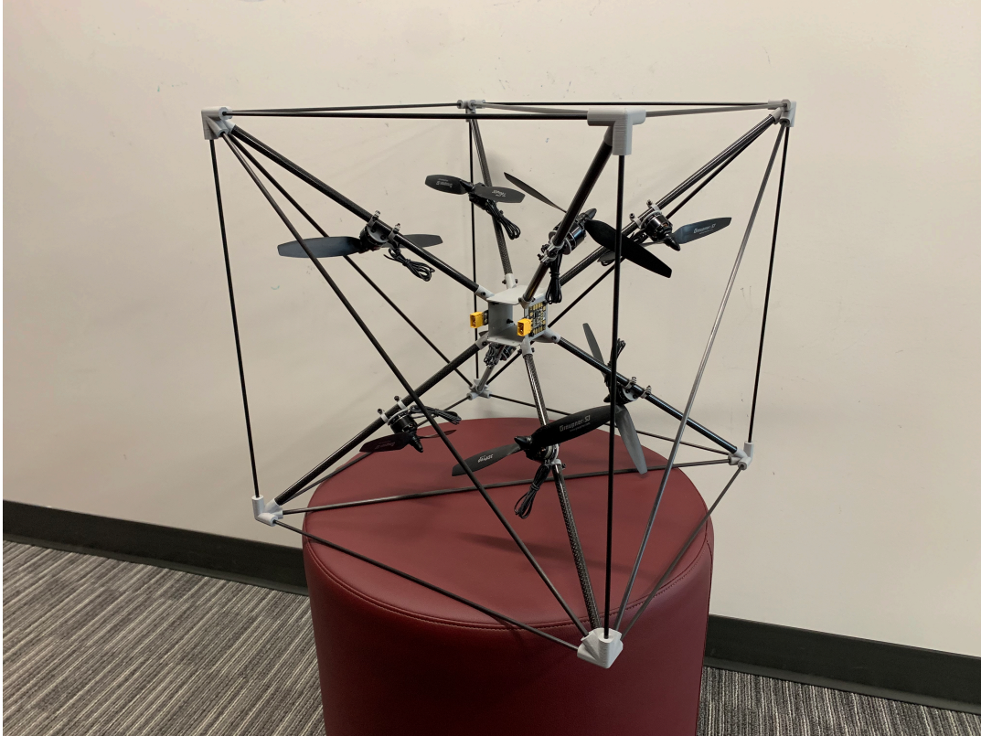
Figure 4.6: Current Omnicopter construction progress, showing the fully assembled vehicle chassis, 3D printed components, and motors mounted in the correct orientations.
