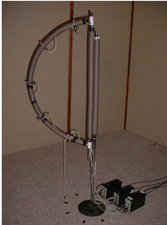
Figure 4.3: Spherical test setup with 5 microphones.
