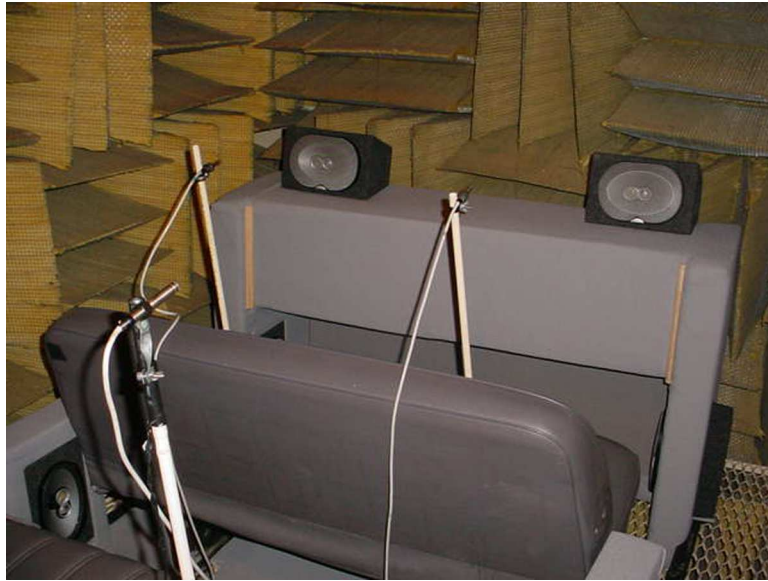
Figure 3.4: Car simulator test setup in anechoic chamber.
