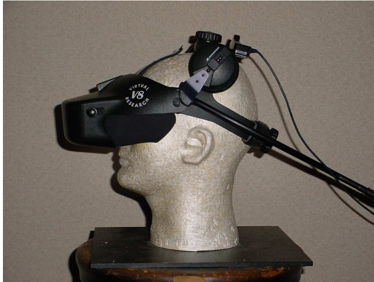
Figure 5.1: Head mounted display used for psychological testing of virtual acoustic environments.
