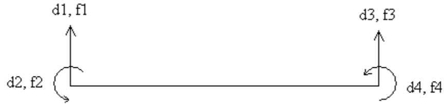
Figure 6.1 Forces on a Typical Beam Element.
