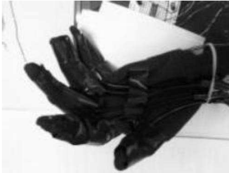
Figure 2.2: Piezoelectric film-based keyboard glove
