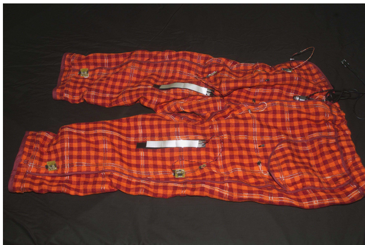
Figure 3.8: Finished e-textile pants prototype (shown inside-out)
