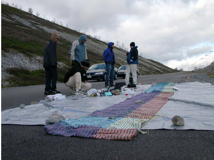
Figure 2.1: Field test of a 30 foot acoustic beamforming textile
