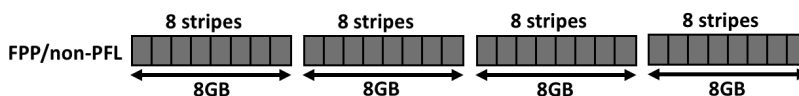
Figure 7.6: Layout in FPP mode - 4 processes each writing 8GB in a non-PFL setup.
