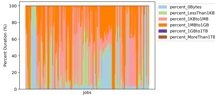
Figure 3.13: Percent I/O duration vs vs size of write bursts.
