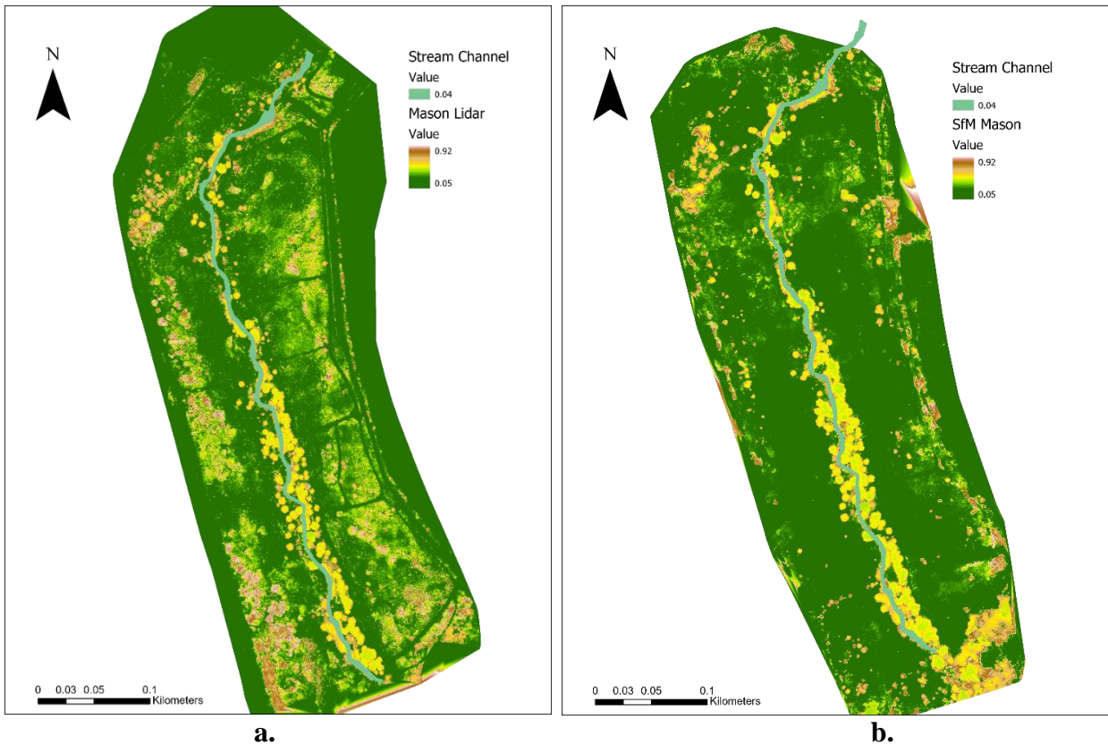
Figure 19. (a) The distribution of spatial roughness determined using the DLS Mason method and (b) distribution of spatial roughness using the SfM Mason method.
