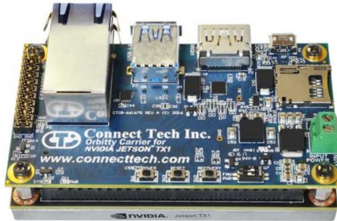
Figure 4.6: Jetson TX2i with Orbitty[16]
