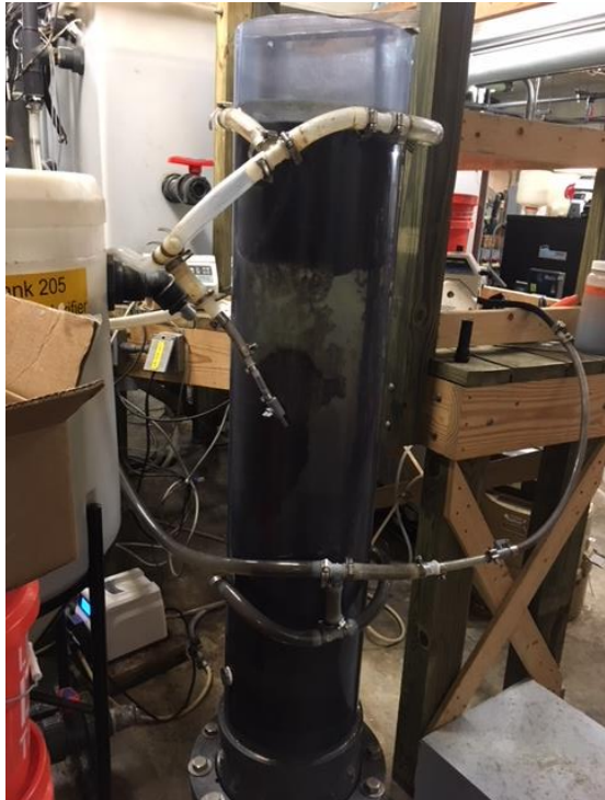
Figure 10: Column photograph shows influent flow combining with internal recycle flow.
