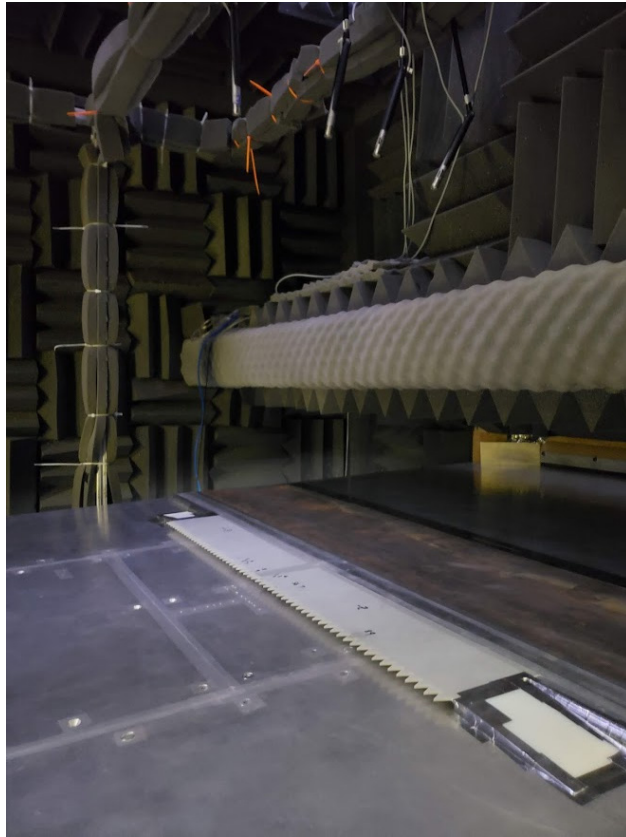
Figure 2.29, Serrated trailing edge and far field microphones in wall jet.
