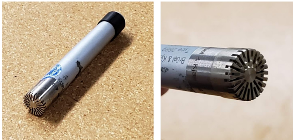
Figure 2.3, B&K Type 4190 1/2" microphone-preamplifier unit.
