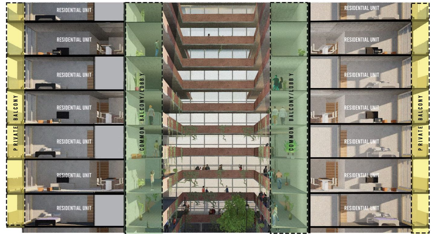
Courtyard Section with Highlighted Balconies
