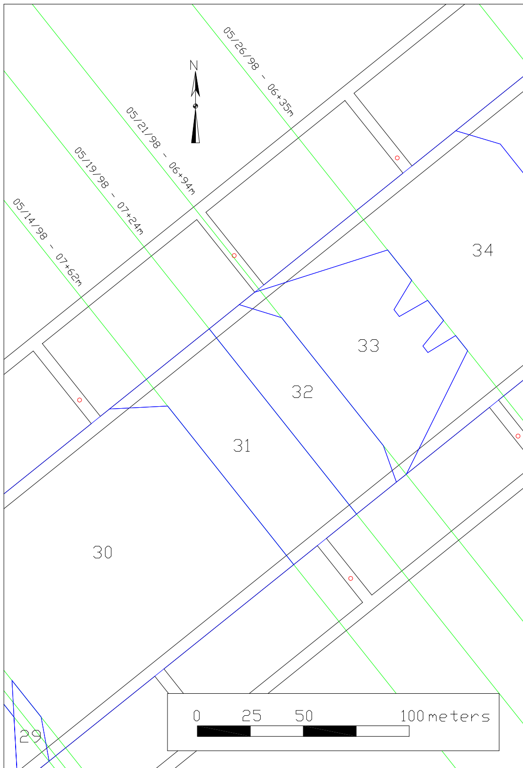
Figure A.6. Plan View of Moonee Colliery Longwall with face locations in green, receivers in red, and falls outlined in blue and numbered.
