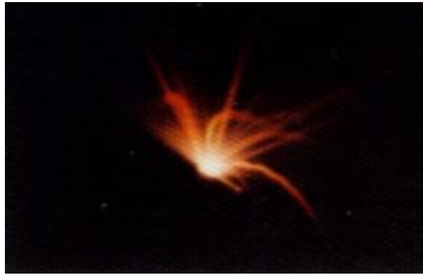
Figure 50: Picture of laser ablation with 1.17 eV Nd:YAG line. The picture shows thermally emitting cadmium and sulfide particles emerging from the target.
