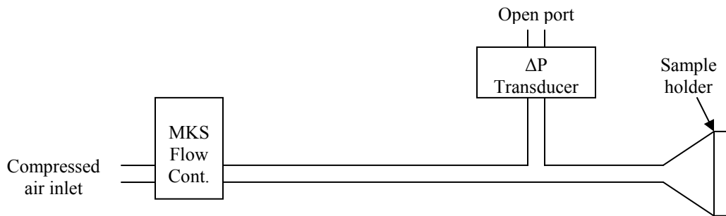
Figure 4.6 - Diagram of through-plane permeability measurement apparatus.
