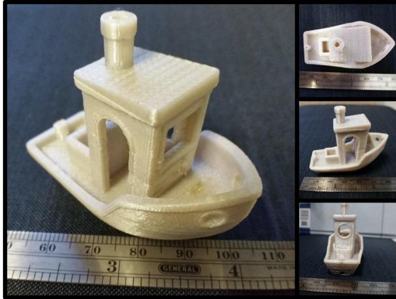
Figure 42: A standard part (3D Benchy) was printed to demonstrate the ability to print more complex parts in the inverted high temperature system.
