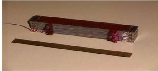
Figure 2.3: Prototype Actuator for INSTAR (Brei et al, 2003)
