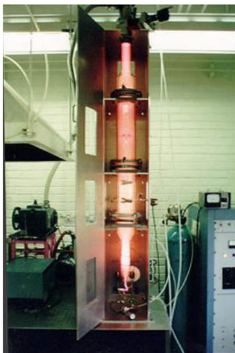
Figure 3.3: Photograph of plasma reactor 1.
