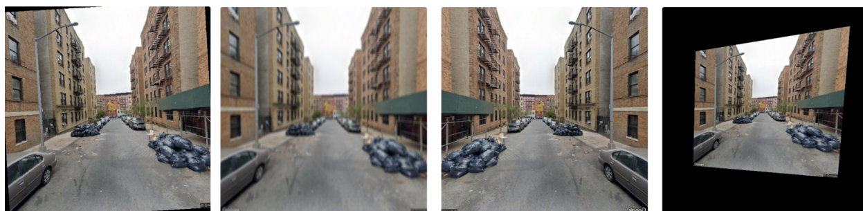
Figure 3.2: Image augmentations were applied to a Google Street View (GSV) image containing two piles of garbage bags from Bronx County, New York. From left to right, the first image augmentation applied was a rotation of 15 degrees. The second image is the result of applying Gaussian blur. The next image is a horizontal flip. Finally, the last image contains a distortion.
