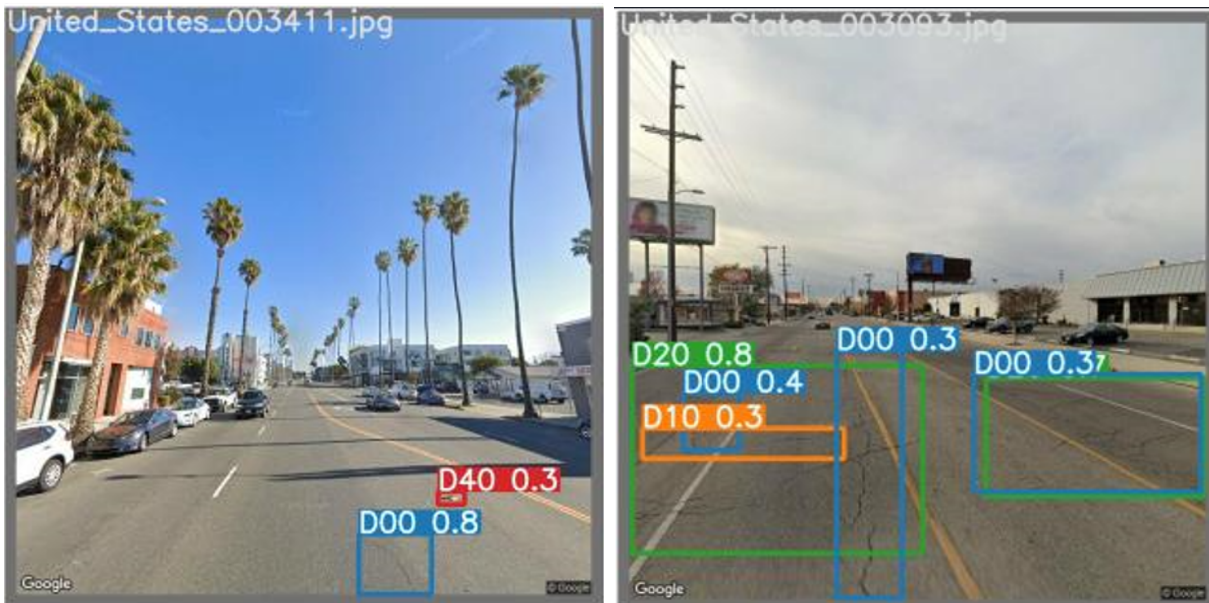
Figure 2.6: The images showcase two Google Street View (GSV) images. Each image was evaluated by a trained YOLOv7 model. The predictions are tagged by a category followed by a confidence score. The labels displayed D00, D10, D20, and D40 are respectively longitudinal cracks, transverse cracks, alligator cracks, and potholes.
