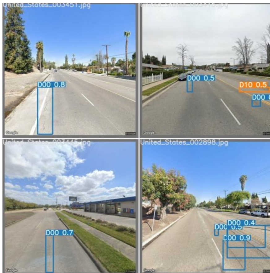
Figure 1.1: The Google Street View images show four distinct roads across the United States. In each image, we observe an object detection model making a prediction on the different types of road damage present. The predictions are tagged by a category followed by a confidence score. D00 represents longitudinal cracks and D10 transverse cracks
