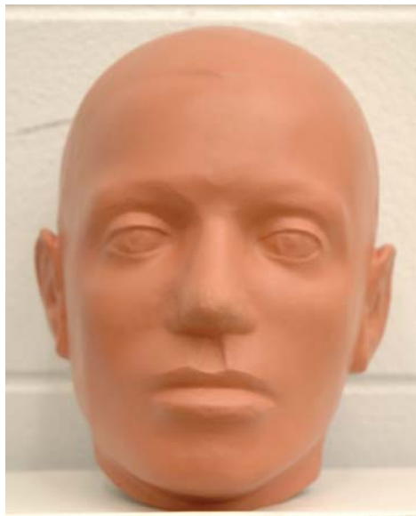
Figure 5: The ANSI headform has the correct anthropometric features for testing eye and face protection, but no instrumentation for measuring impact forces.
