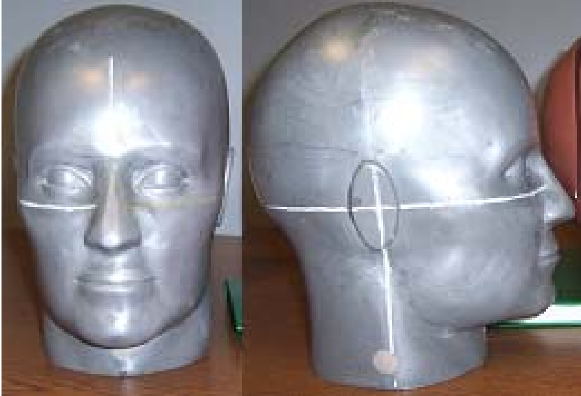
Figure 6: The USAARL headform models the 50 th percentile tri-services soldier facial anthropometry.
