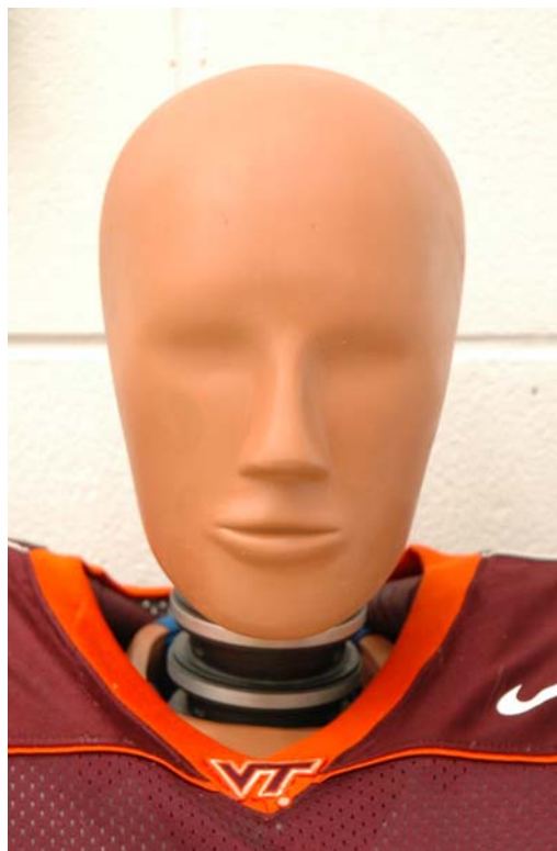
Figure 4: The Hybrid-III headform lacks detailed facial features.
