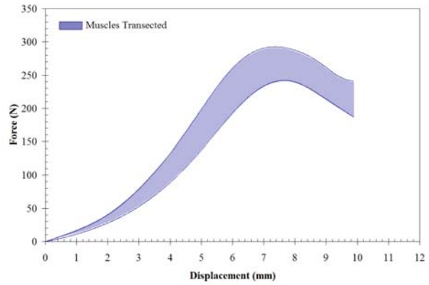
Figure 19: Force-deflection corridors generated from the five in-situ eye impact tests with extraocular muscles transected.
