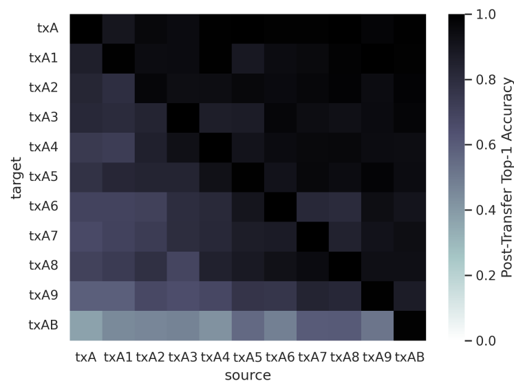
Figure 25. The post-transfer top-1 accuracy for each source/target dataset pair constructed for the Captured Model Refinement SEI experiment using fine-tuning, shown on a scale of [0.0, 1.0].
