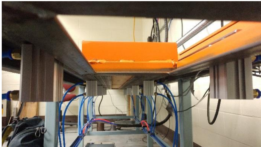
Figure 3-17: 10 Pneumatic cylinders for raising the track. The cylinder housing is bolted to the bottom of the table, and the cylinder is free to pass through holes in the table, moving the linear guides and carriage upward.
