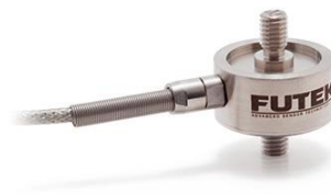
Figure 3-14: Futek sensor for measuring the friction force
