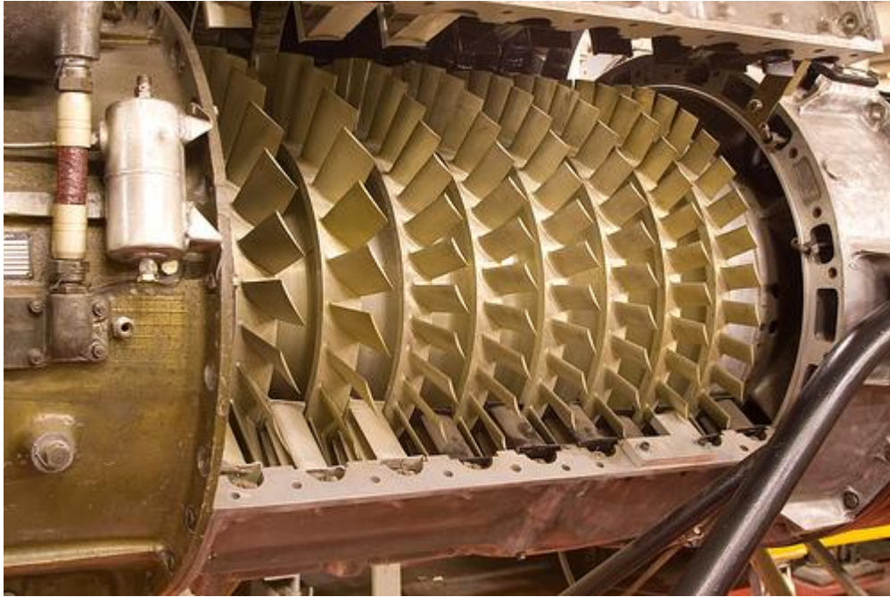
Figure 1.1.2: Multistage Axial Compressor
