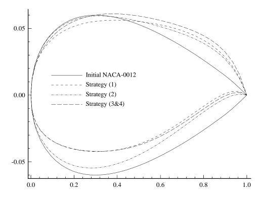
Figure 6.3: Initial and final optimized airfoil surfaces for each strategy.
