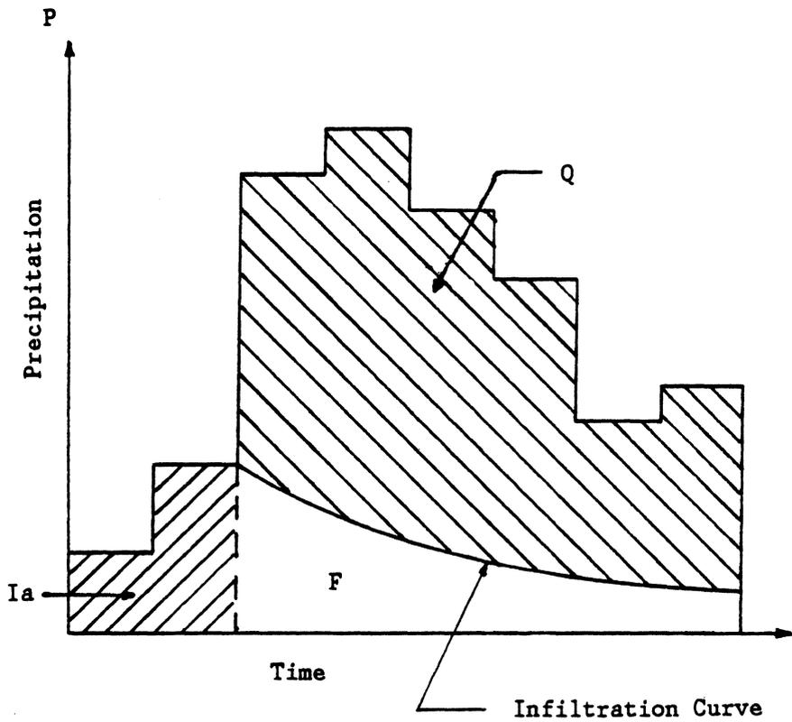
Figure 2. Relationship Between Precipitation, Runoff, and Retention (SCS TR - 55, 1975)
