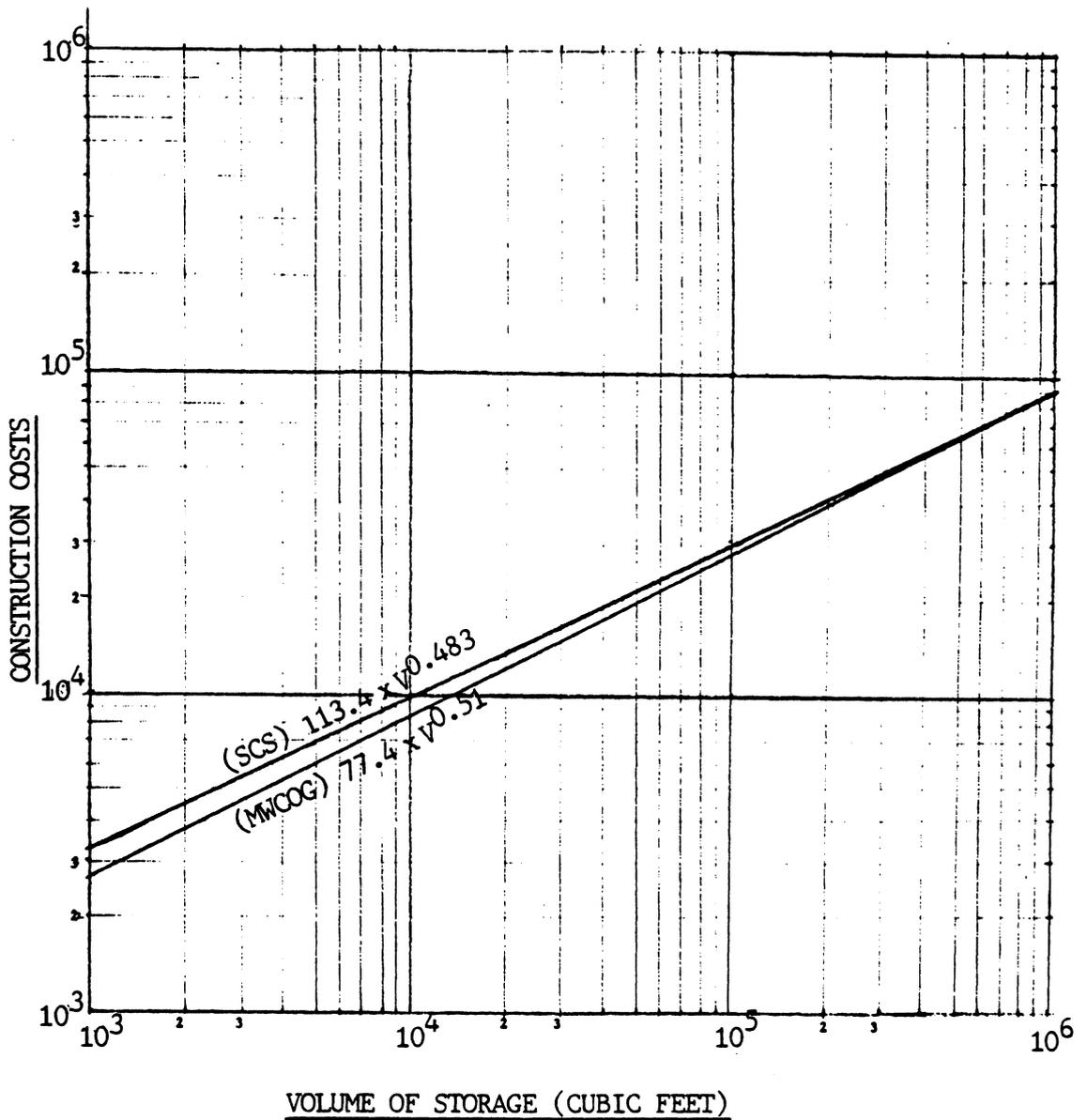
Figure 8. Relationship Between Detention Pond Construction Cost and Storage Volume (MWCOG 12-82)
