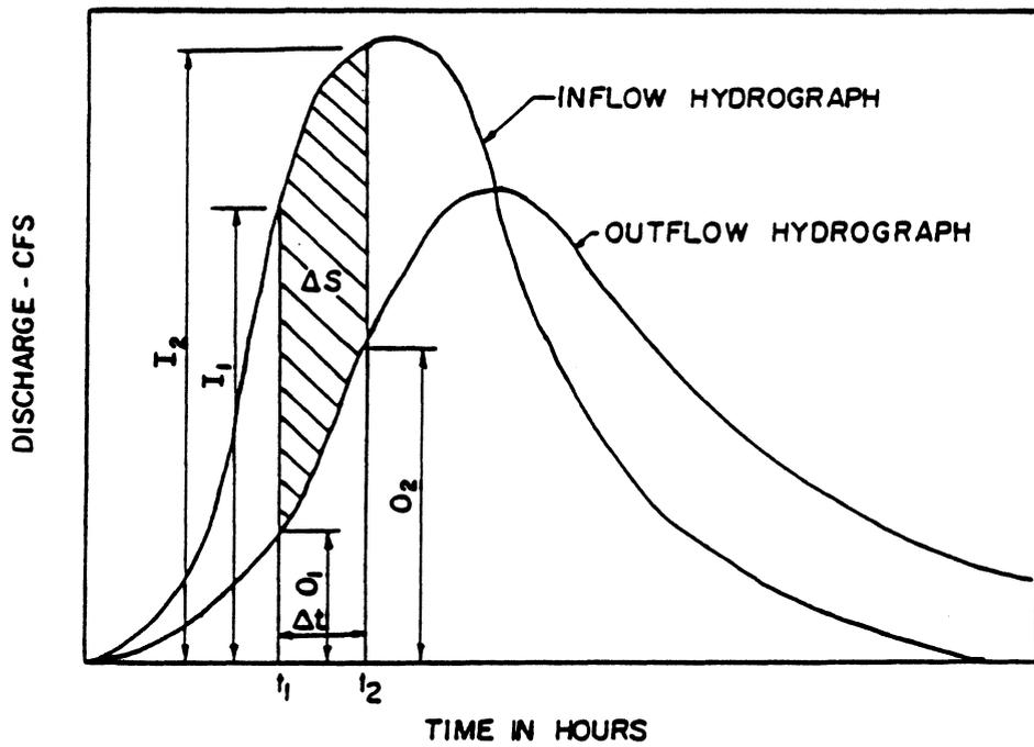
Figure 4. Derivation of Storage for Storage - Indication Working Curve Method
