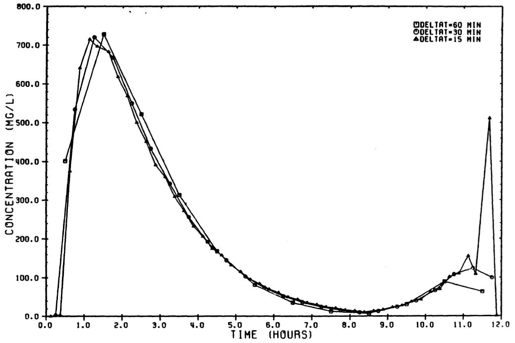
Figure 10. Pollutograph Time Increment Sensitivity--Total Suspended Solids
