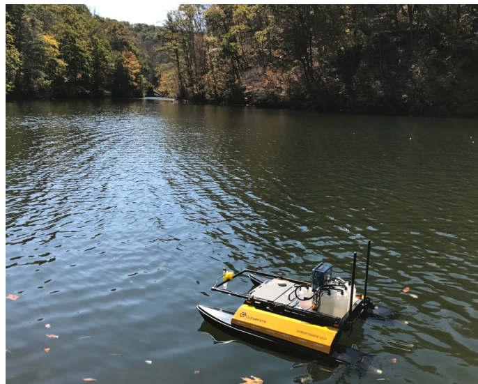
Figure 3.2: The Clearpath Robotics Kingfisher USV equipped with the automated water sampler on Claytor Lake, VA, USA. The water sampler onboard the USV collected samples of water at two different depths. Each sample was collected into sterile 1 L bottles. The operation of the vacuum pumps and sampling tubes were remote-controlled through a microcontroller and supporting electronics housed in a waterproof box. A collection bottle containing 500 mL of sterile water was used as an unexposed control during each mission. Image courtesy of D. Schmale.
