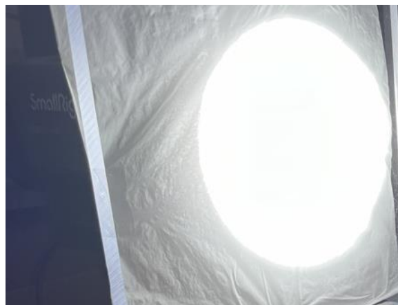
Figure 11: Acrylic Block with Diffuser Paper in Front of Light.
