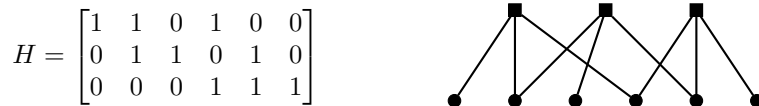
FIGURE 1. A parity check matrix H (left) for a linear code and its corresponding Tanner graph T(H) (right). Here and throughout, variable nodes are represented with circles and check nodes are represented with squares.
