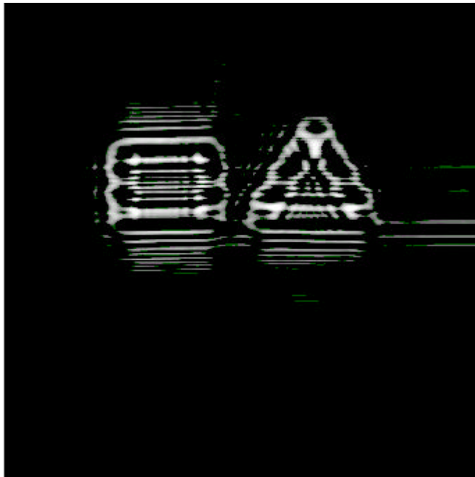
Figure (5.2-4b): Sine- hologram of a 3-D target object with different depth location but otherwise the target object is the same as the 3-D reference object.
