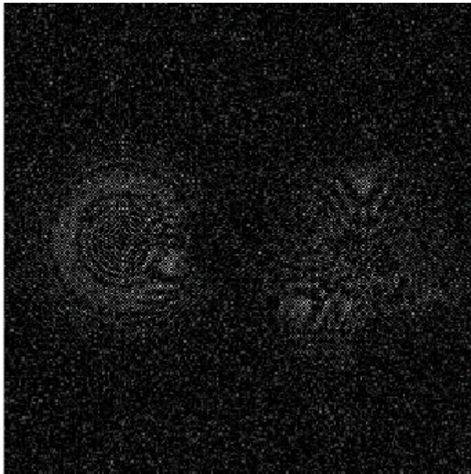
Figure (4.3-16a): Cosine-FZP hologram of the 3-D target object shown in fig. (4.3-7) in the presence of noise.
