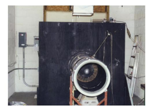
Figure 3.4: Photo of Bellmouth, Inlet Duct, and Plenum Chamber.
