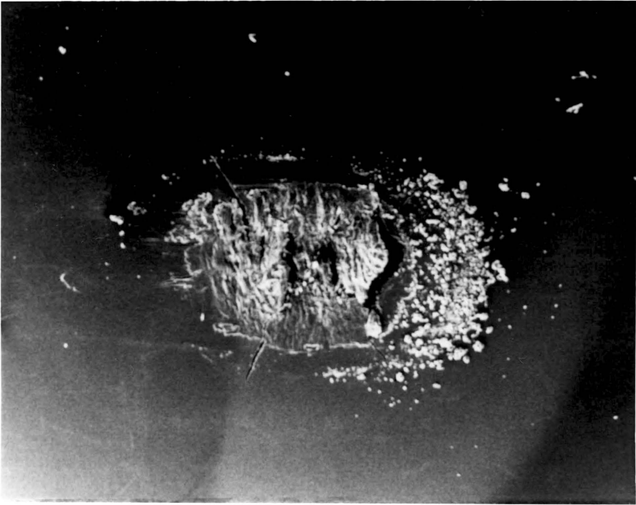
FIGURE 4-74. Scanning Electron Micrograph of PS Test 1 Disk Scar (Magnification: 20X).
