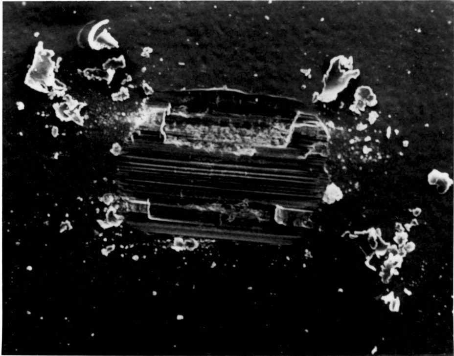
FIGURE 4-34. Scanning Electron Micrograph of PI Test 1 Disk Scar (Magnification: 50X).
