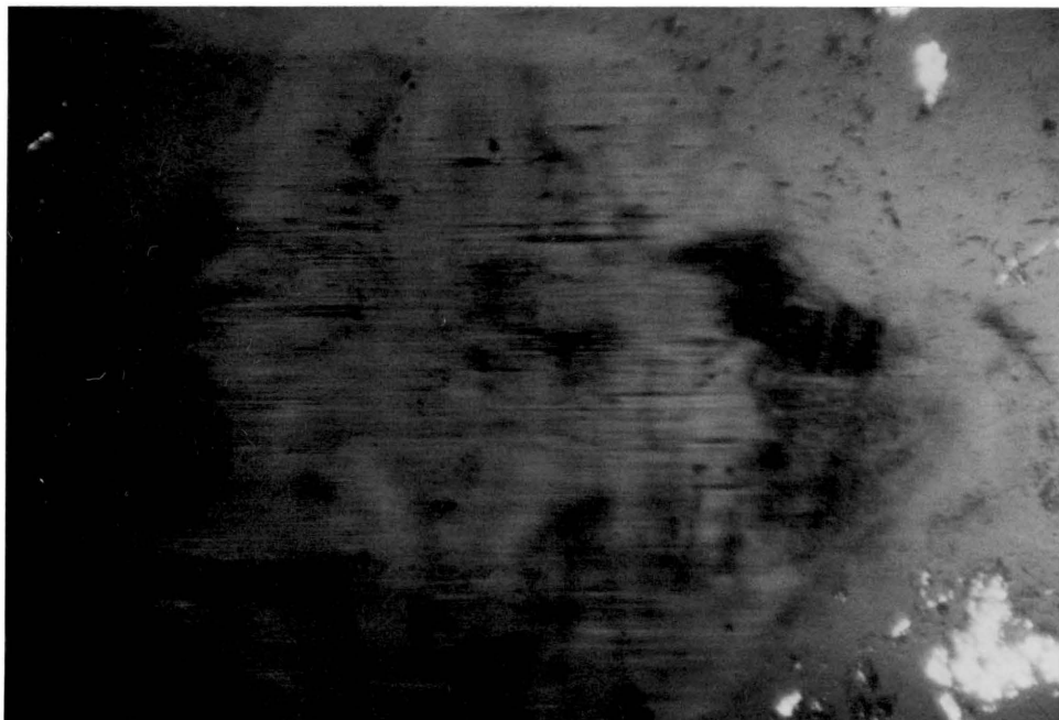
FIGURE 4-63. Optical Macrograph of PSO Test 1 Ball Scar (Magnification: 60X).
