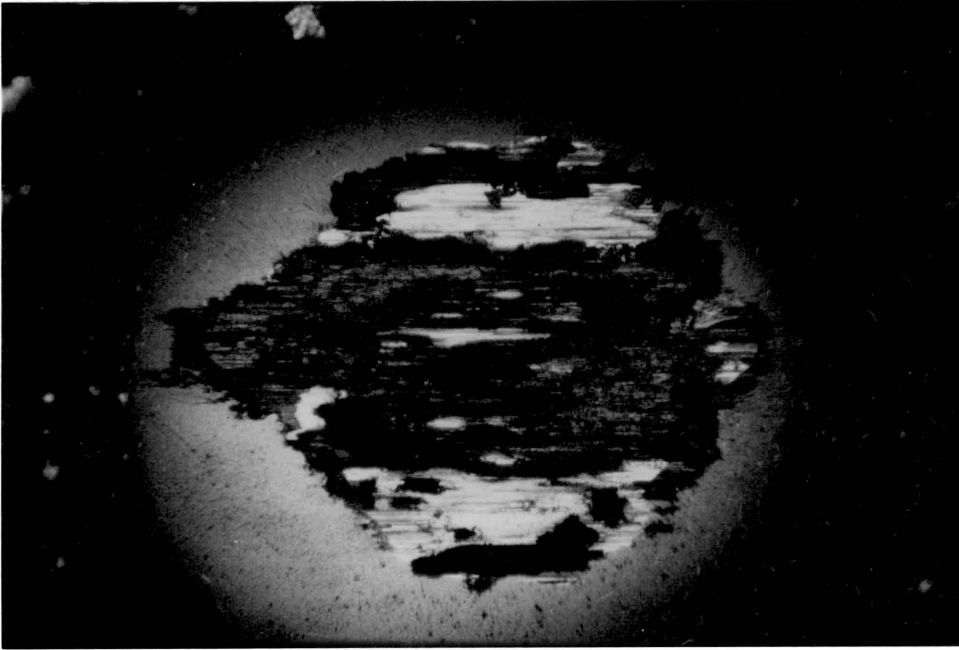
FIGURE 4-36. Optical Macrograph of PI Test 3 Ball Scar (Magnification: 37.5X).
