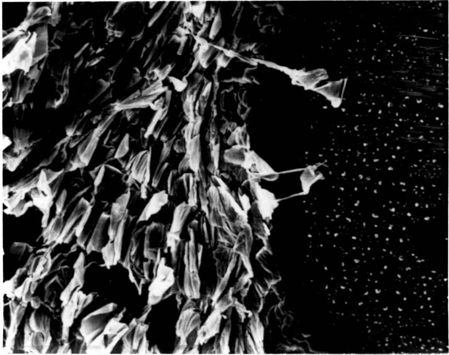
FIGURE 4-31. Scanning Electron Micrograph of PTFE Test 3 Disk Scar End (Magnification: 200X).
