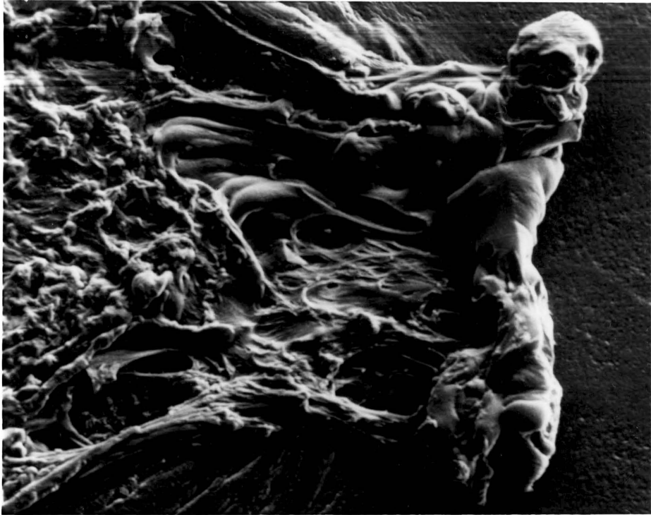
FIGURE 4-47. Scanning Electron Micrograph of PVDC Test 1 Disk Scar (Magnification: 200X).
