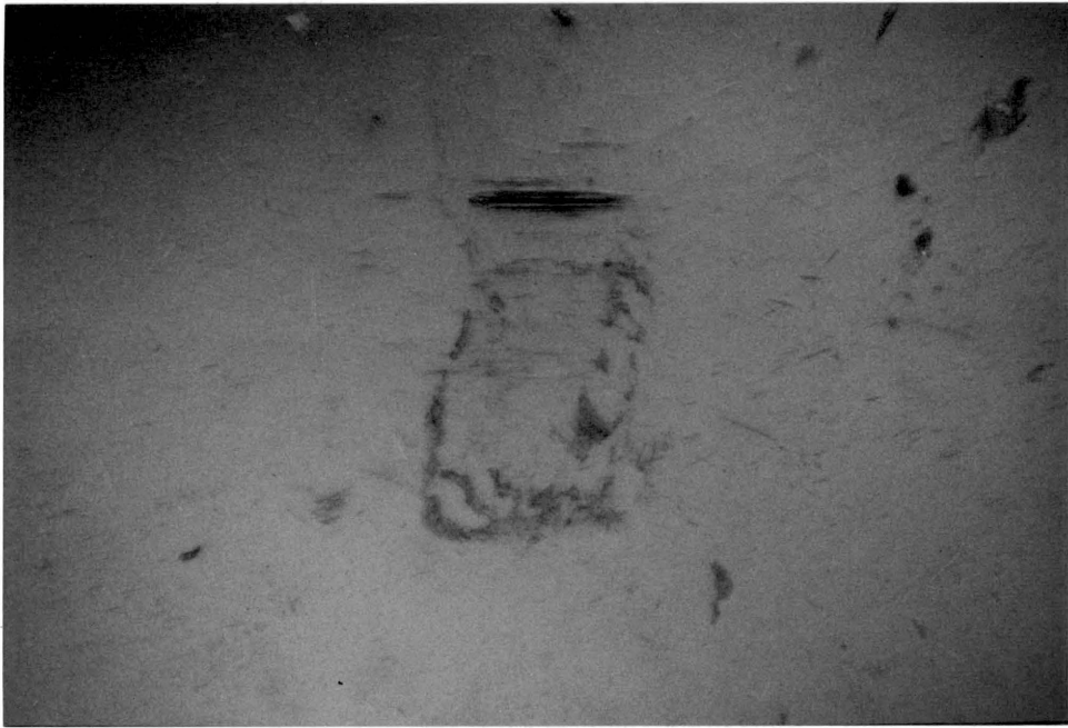
FIGURE 4-24. Optical Macrograph of PMMA Test 3 Disk Scar (Magnification: 60X).
