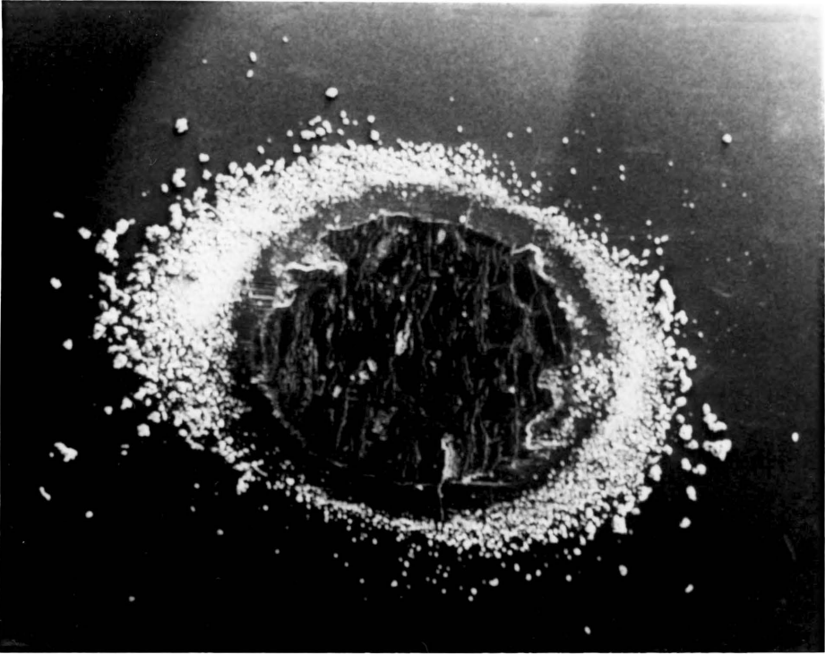
FIGURE 4-78. Scanning Electron Micrograph of PS Test 3 Disk Scar (Magnification: 20X).
