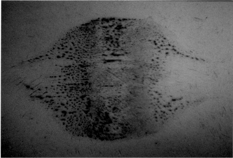
FIGURE 4-44. Optical Macrograph of PVDC Test 1 Ball Scar (Magnification: 60X).
