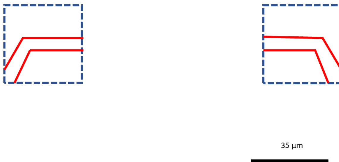
Figure C.2: The outline used with NPGS software to perform the alignment between macroscopic electrodes and nanoscale features, as described in Chapter 2.
