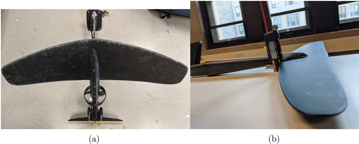
Figure 2.2: (a) Trapezoidal fore foil with span wise anhedral curve, (b) Trapezoidal aft foil with maximum thickness of 1 cm
