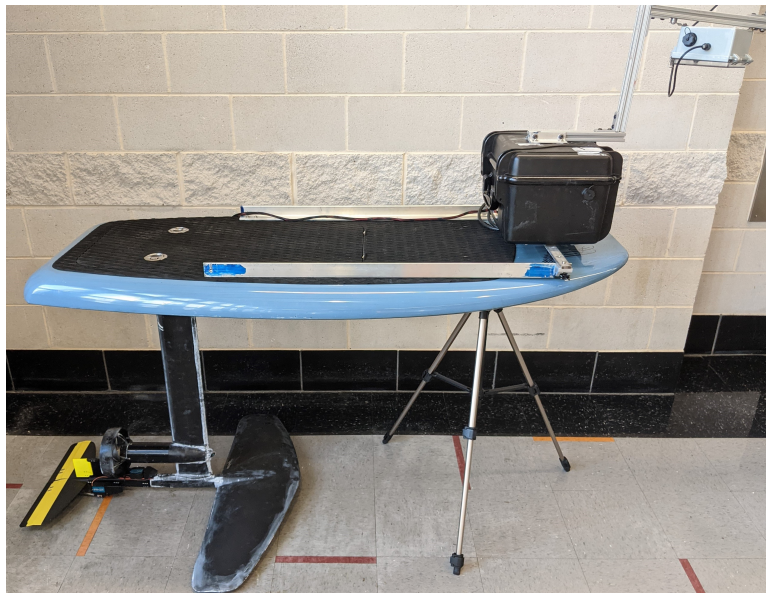
Figure 2.1: eFoil from Lift Foils modified with control flaps and additional electronics for autonomous operation
