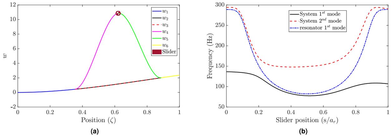
**Figure 3.** (a) The first mode of the combined structure at slider position  $s = 0.5a_r$ ; different systems' portions highlighted in the supplementary material (i.e.,  $w_i$  are demonstrated in the legend in addition to the slider); however, the y-axis represents the structure displacement (i.e.,  $w$ ); (b) comparison between the combined structure mode shapes and the resonator at different slider positions.
