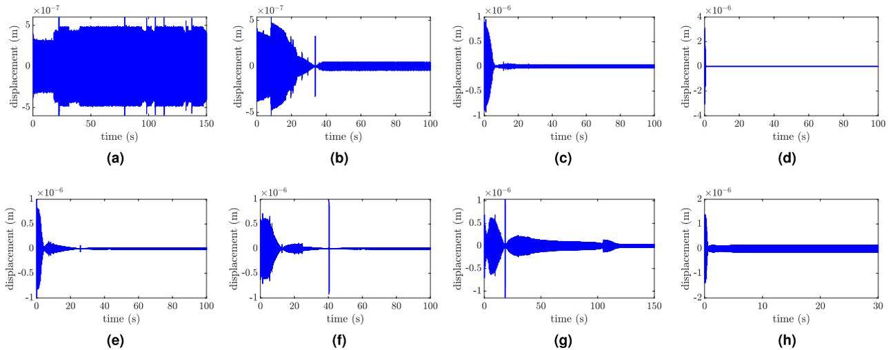
**Figure 6.** Tip displacement of the primary structure at different excitation frequencies: (a)  $f = 78$  Hz,  $w_0 = 0.1g$ ; (b)  $f = 85$  Hz,  $w_0 = 0.1g$ ; (c)  $f = 130$  Hz,  $w_0 = 0.1g$ ; (d)  $f = 140$  Hz,  $w_0 = 0.1g$ ; (e)  $f = 150$  Hz,  $w_0 = 0.1g$ ; (f)  $f = 155$  Hz,  $w_0 = 0.1g$ ; (j)  $f = 200$  Hz,  $w_0 = 0.5g$ ; (h)  $f = 250$  Hz,  $w_0 = 0.8g$ .
