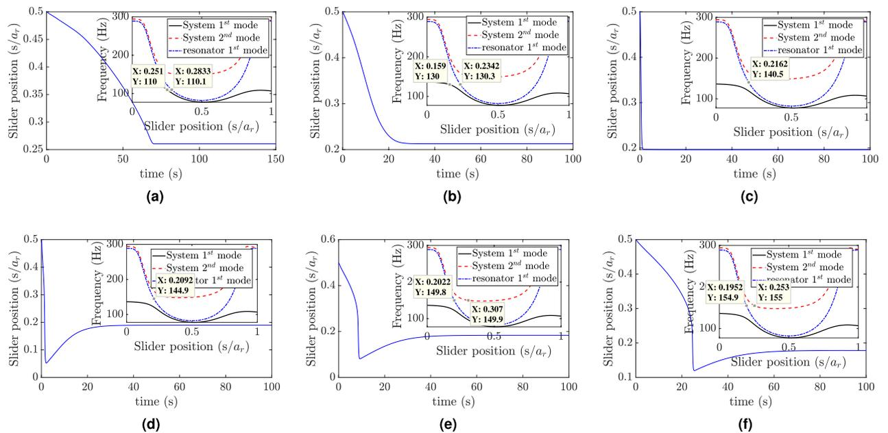
**Figure 7.** Slider position at different excitation frequencies: (a)  $f = 110$  Hz,  $w_0 = 0.1g$ ; (b)  $f = 130$  Hz,  $w_0 = 0.1g$ ; (c)  $f = 140$  Hz,  $w_0 = 0.1g$ ; (d)  $f = 145$  Hz,  $w_0 = 0.1g$ ; (e)  $f = 150$  Hz,  $w_0 = 0.1g$ ; (f)  $f = 155$  Hz,  $w_0 = 0.1g$ .
