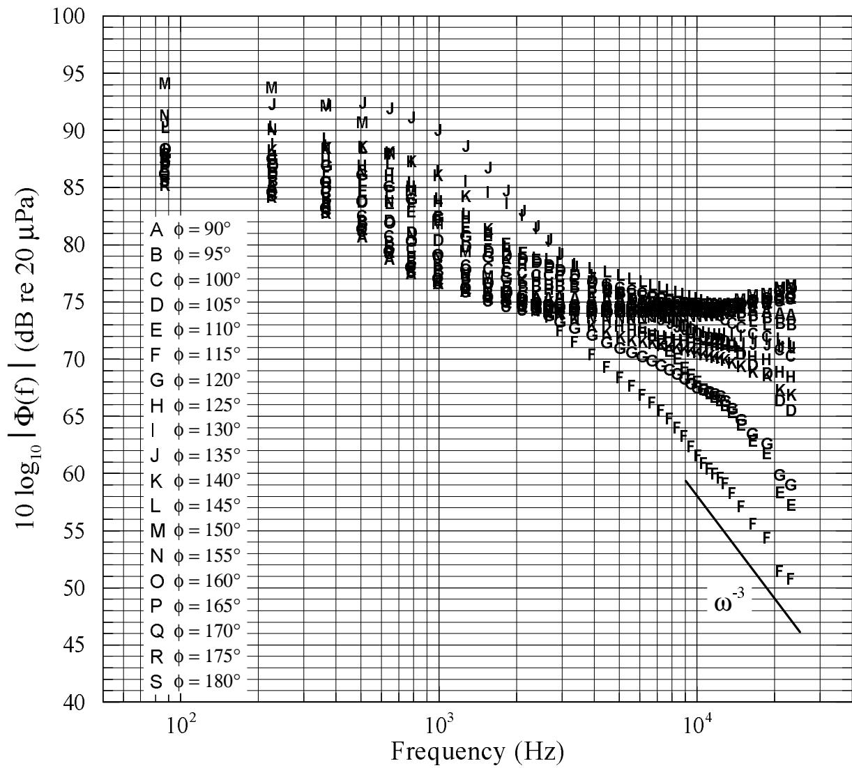
**Figure 119.** Power spectra of surface pressure fluctuations at  $\alpha = 20^\circ$ ,  $x/L = 0.772$ .
