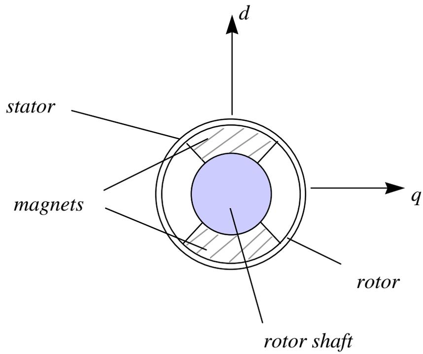
Figure 3.  $DQ$  axis orientation in a two pole PMSM
