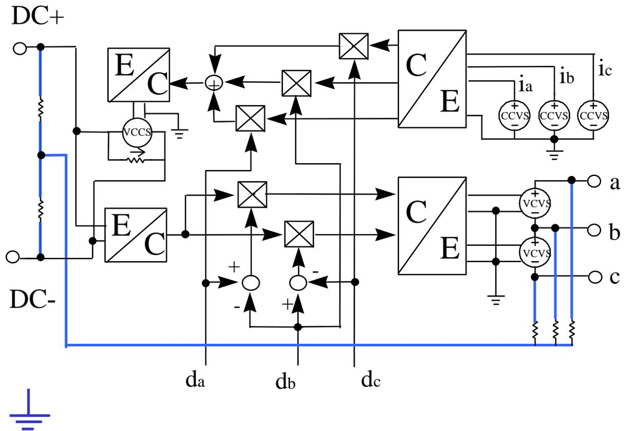
Figure 9. VSI three-phase average modeling - signal transformations
