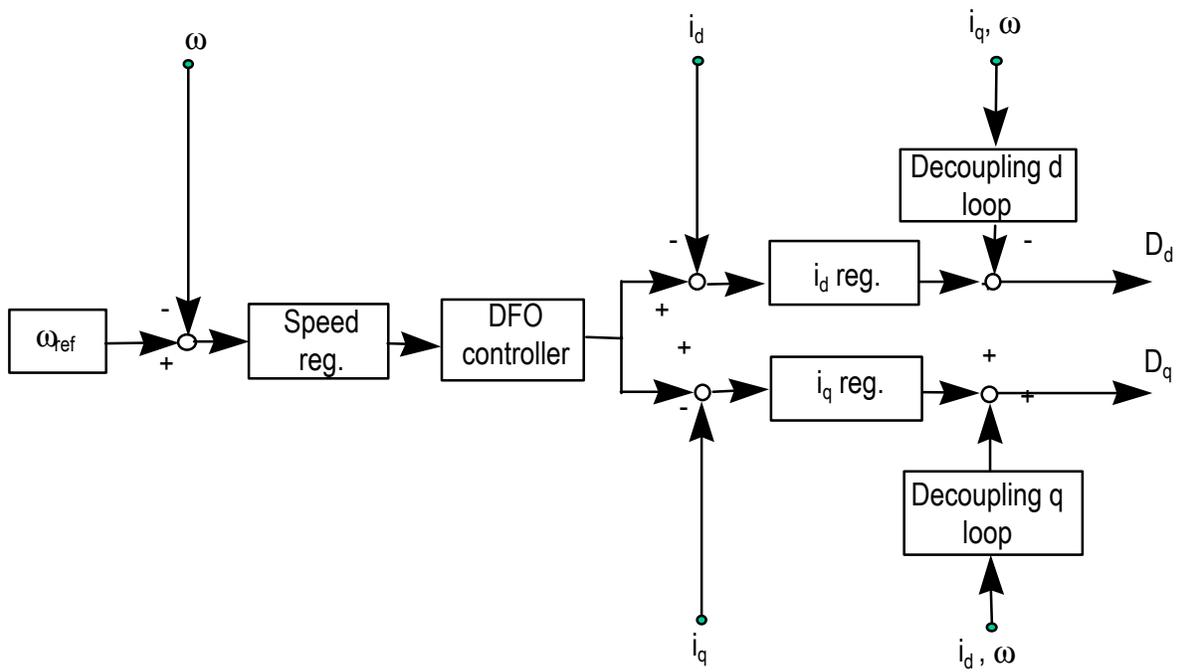
Figure 6. Two-stage cascade controller module model
