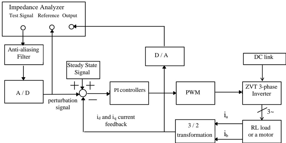
Figure 11. Measurement scheme for current loop transfer functions
