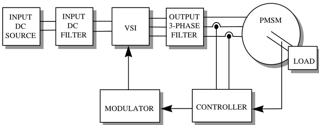
*Figure 1. Block diagram of a VSI fed PMSM drive*
