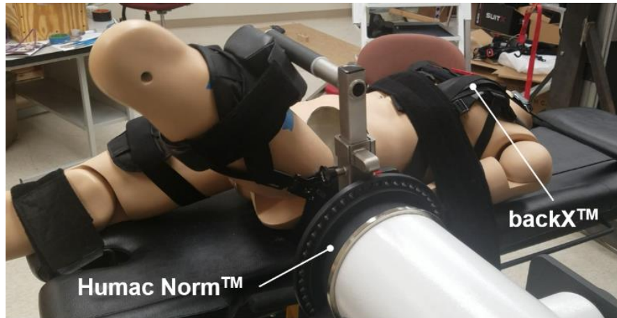
Figure 4-1. Demonstration of the torque profile measurements for the backX™ using a dynamometer.
