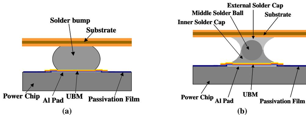
Figure 2.30. (a) Single bump solder joint structure; (b) Triple-stacked high standoff solder joint structure.
