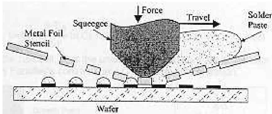
Figure 2.33. Stencil printing process for solder deposition [49].
