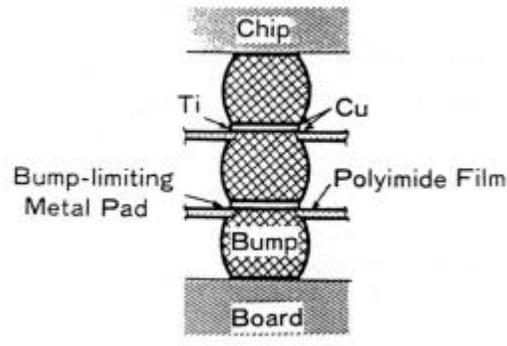
Figure 2.20. Stacked solder-bump interconnection [18]
