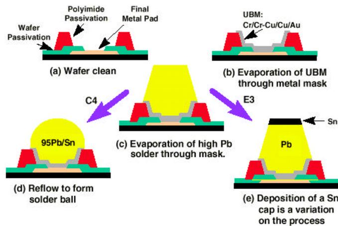
Figure 2.3. Evaporative Solder Bumping Process [1].
