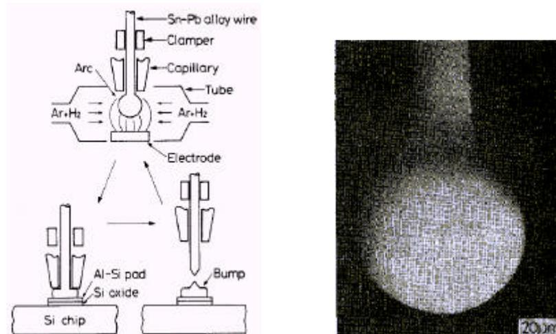
Figure 2.9. (a) Some fundamental motions for solder bump formation and (b) SEM photo of the solder alloy ball formed by arc discharge [10].
