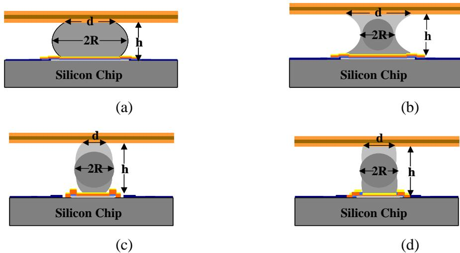
Figure 2.31. Cross section schematics of the dimension parameters of four solder joint structures, (a) Single bump barrel shape; (b) Triple-stacked hourglass shape; (c) Triple-stacked barrel shape; and (d) Triple-stacked column shape.
