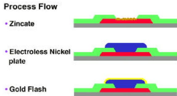
Figure 2.11. Zincation enables the electroless plating of nickel on top of the aluminum bond pad [1].
