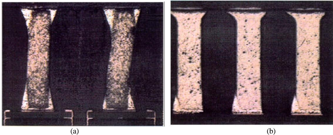
Figure 2.23. Cross sections of wire (a) and cast (b) CCGAs after initial card attach [23].
