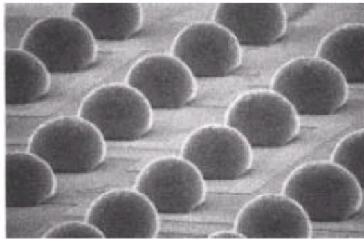
Figure 2.7. Solder bumps on wafer [7].
