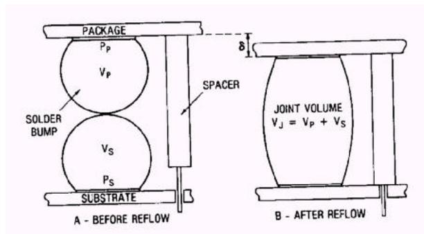
Figure 2.21. Double-bump assembly process [20]
