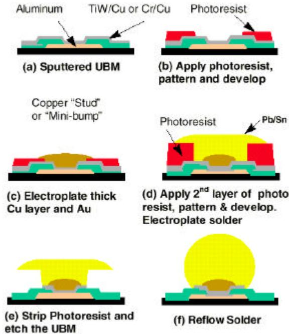
Figure 2.8. Electroplated UBM w/Mini Bump and Solder [8].
