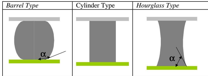
Figure 2.29. Types of common solder joints.
