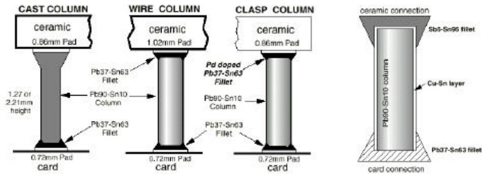
Figure 2.22. Schematic depicting Ceramic Column Grid Array (CCGA) structures assembled to a card [21].
