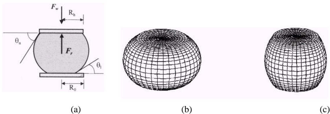
Figure 2.24. (a) Schematic of a solder ball subjected to an external load; (b) First and (c) second reflow geometry of the solder ball in a BGA assembly [19].
