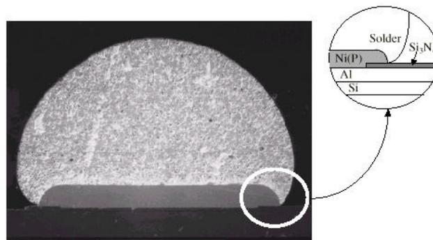
Figure 2.13. Scanning electron micrograph of an electroless nickel UBM with eutectic 63Sn/37Pb solder deposited on top [1].
