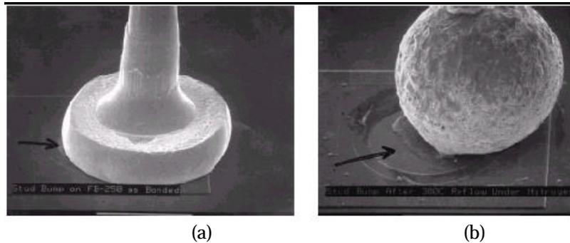
Figure 2.10. (a) SEM micrograph of a Sn/Pb SBB; (b) SEM micrograph of stud bump after 300°C reflow in a nitrogen. Solder has dewetted from the Al bond pad [1].
