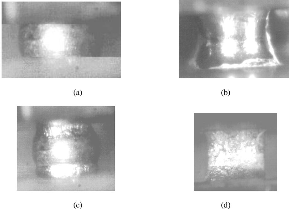
Figure 2.32. Microphotographs of solder joints with different heights and shapes; (a) Single bump barrel-shaped; (b) triple-stacked hourglass-shaped; (c) triple-stacked barrel-shaped; and (d) triple-stacked column-shaped.
