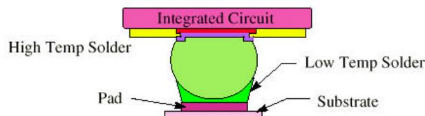
Figure 2.4. High temperature solder joined to non-ceramic substrate [1].
