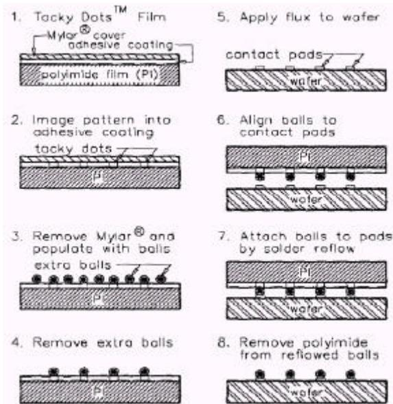
Figure 2.18. Tacky Dots™ assembly flowchart [17].
