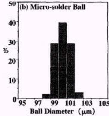
Figure 2.14. Ball size distribution of micro solder balls 100  $\mu\text{m}$  in diameter [13].
