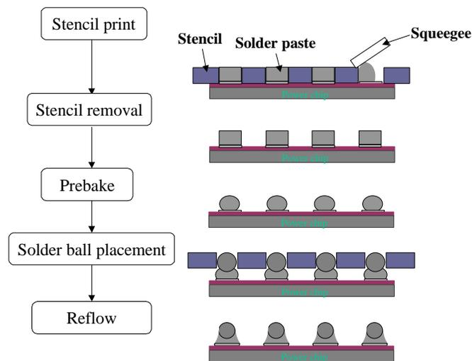
Figure 2.38. Stacked solder bumping process.
