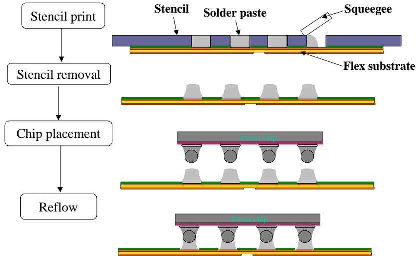
Figure 2.40. Triple-stacked solder bump bonding process.
