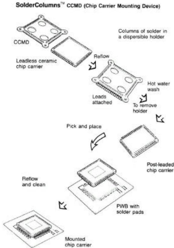
Figure 2.28..Flowchart of chip carrier mounting device assembly process [27].
