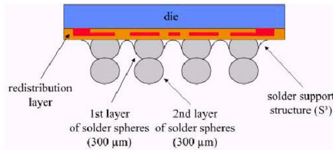
Figure 2.25. Schematic cross section of the S<sup>3</sup>-diepack [25].
