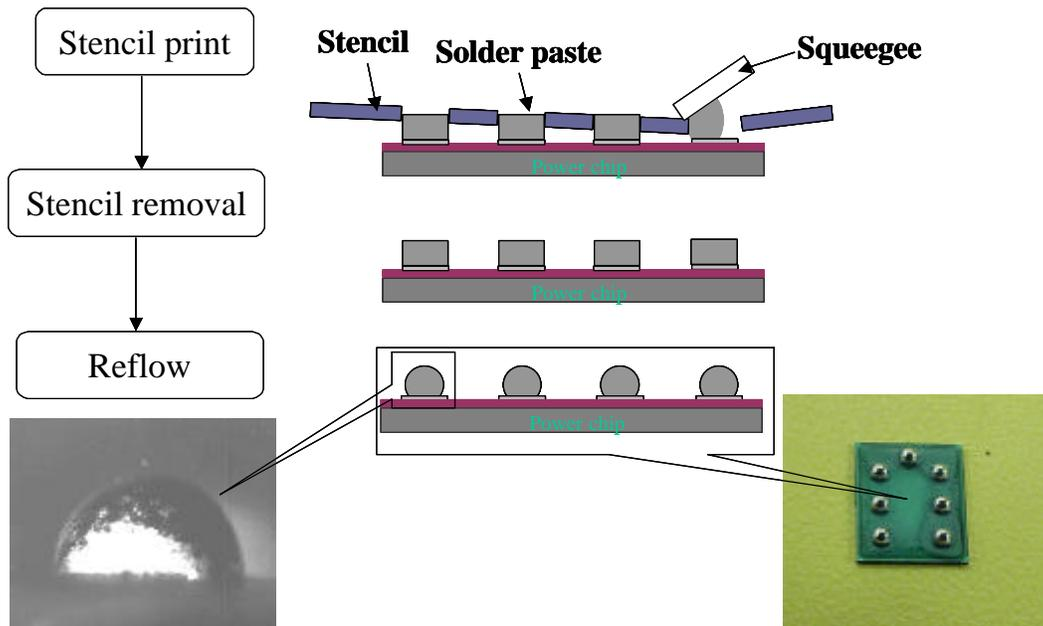
Figure 2.36. Solder bumping process using stencil printing for single bump solder joint fabrication.
