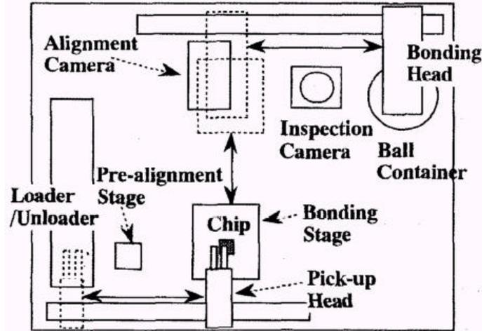
Figure 2.16. Schematic diagram of microball mounter [13].
