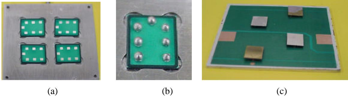
Figure 2.34. Process for solder joint formation on power chip; (a) solder mask patterning; (b) solder bumping; and (c) flip chip bonding.
