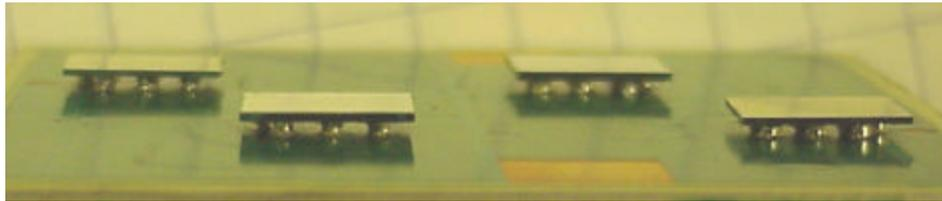
Figure 2.41. Flip chip on substrate assembly before underfill.
