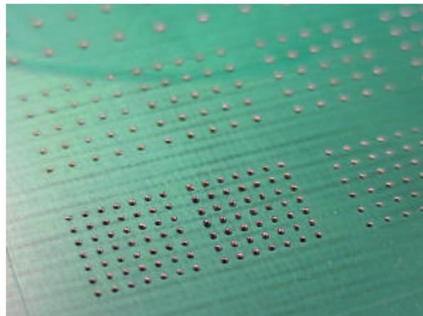
Figure 2.35. Solder joint arrays of different pitch and size.
