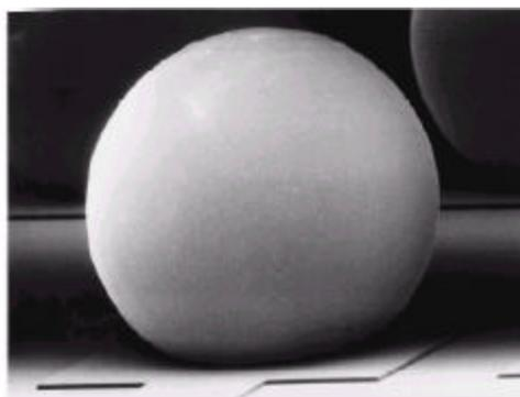
Figure 2.2. Scanning electron micrograph of a eutectic solder bump on a silicon IC [1].
