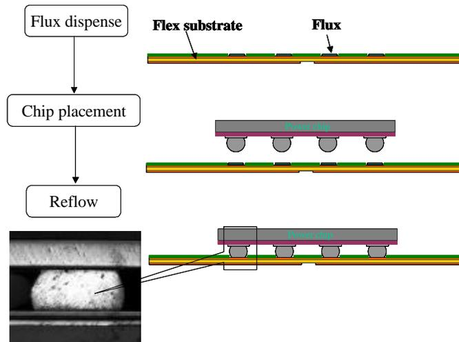
Figure 2.37. Flip chip bonding process for single bump solder joint fabrication.
