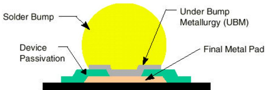
Figure 2.1. Schematic of a solder joint showing the final metal, under-bump-metallurgy and solder ball. These three metals must be joined, forming a single metallurgical system [1].
