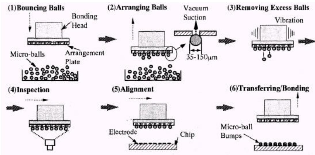
Figure 2.15. Flow chart of the microball arranging and transferring process [13].
