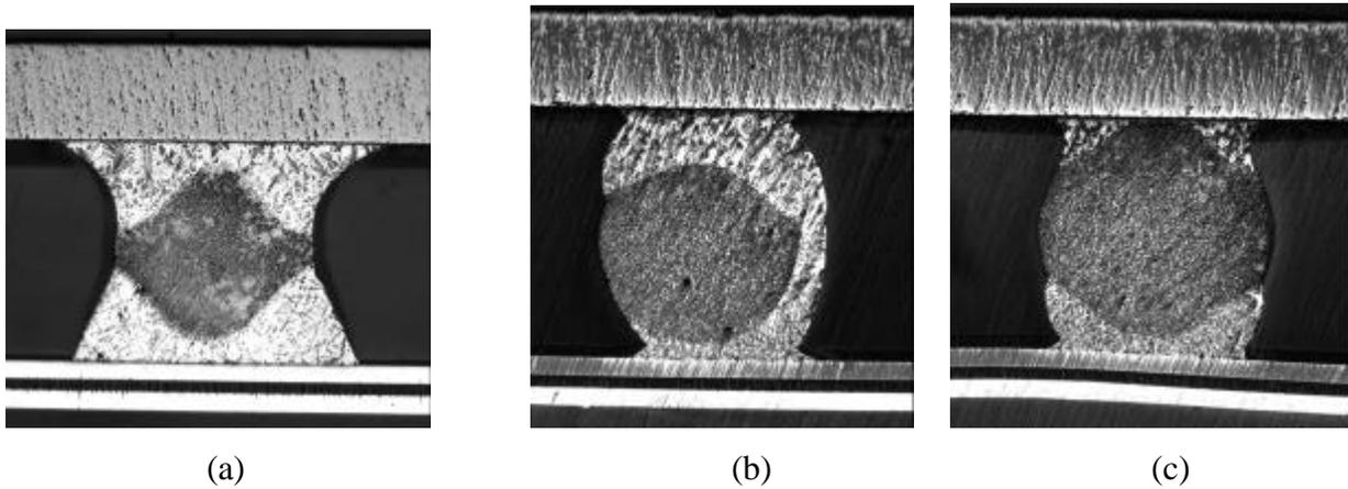
Figure 2.42. Photographs of stacked solder joints; (a) hourglass-shaped; (b) barrel-shaped; and (c) column-shaped.
