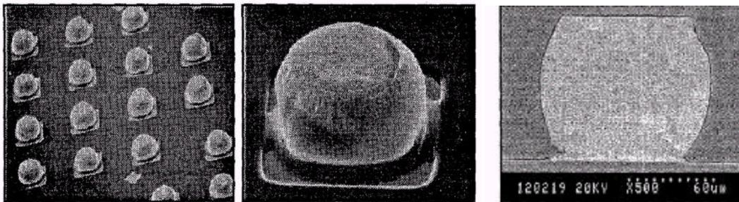
Figure 2.19. Once-reflowed Tacky Dots solder bumps and cross section view [17].
