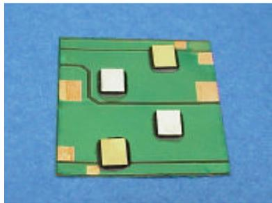
Figure 2.43. Flip chip on flex (FCOF) assembly after underfill.
