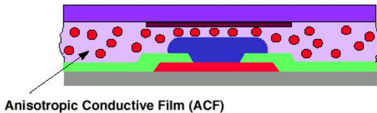
Figure 2.12. Illustration of an electroless nickel UBM assembled to a substrate with conductive adhesive. This produces a very low profile assembly [1].
