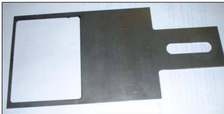
**Figure A.2.** The holder that supports the heat sink and substrate in the e-beam.
