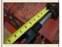
10. Retract hydraulic cylinders. Hydraulic cylinder rods on implements are subject to pit corrosion, or pits in the metal, if left extended and stored outside for a season. Pit corrosion can tear out the seals on the cylinders the next time you use the implement. You should retract the cylinders or coat the rods with heavy grease to protect them.
