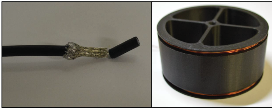
Figure 22: Left - Probe made for field mapping, Right-Helmholtz coil made to calibrate the new probes
