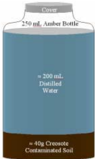
Figure 4.2 Schematic of batch experiment
