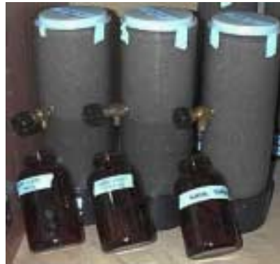
Figure 4.9 Soil column drainage technique
